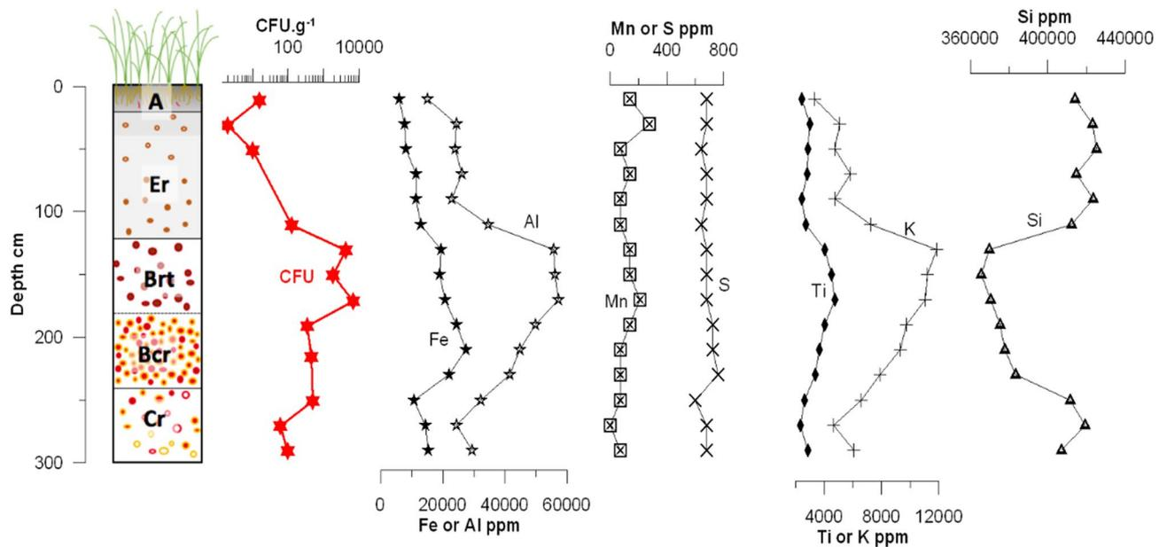
**Figure 6.** Soil log showing the main pedological horizons (i.e. A, Er, Brt, Bcr and Cr—see caption of Fig. 4 for meaning of abbreviations), semi-quantitative colony forming unit (CFU) counts of *B. pseudomallei* (CFU g<sup>-1</sup>), and elemental concentration along the 300-cm deep profile: iron (Fe), aluminum (Al), manganese (Mn), sulfur (S), titanium (Ti), potassium (K), silicium (Si).
