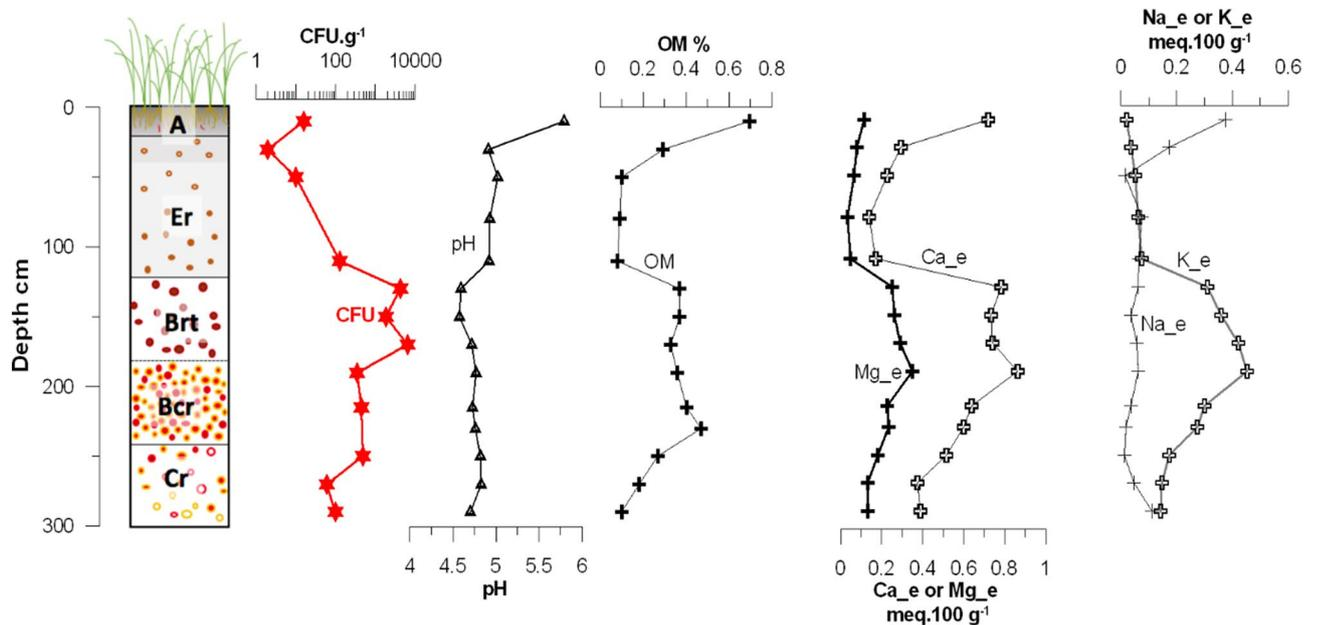
**Figure 5.** Soil log showing the main pedological horizons (i.e. A, Er, Brt, Bcr and Cr—see caption of Fig. 4 for meaning of abbreviations), semi-quantitative colony forming unit (CFU) counts of *B. pseudomallei* (CFU g<sup>-1</sup>), and soil physico-chemical parameters along the 300-cm deep profile: pH, organic matter content (OM), exchangeable magnesium (Mg<sub>e</sub>), exchangeable calcium (Ca<sub>e</sub>), exchangeable sodium (Na<sub>e</sub>) and exchangeable potassium (K<sub>e</sub>).
