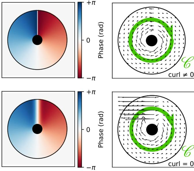
**Fig. 6.** Schematic for the gradient measured by a SH for a sharp discontinuity (*top*) and for a smoother pattern (*bottom*). In the top case, the amplitude of the discontinuity is not estimated correctly, and consequently the sum of SH slopes along a closed path  $\mathcal{C}$  is not equal to zero. In the bottom case, the sum of slopes along the path  $\mathcal{C}$  is equal to zero because the strong slope in affected subapertures compensate exactly for the rest of the path.
