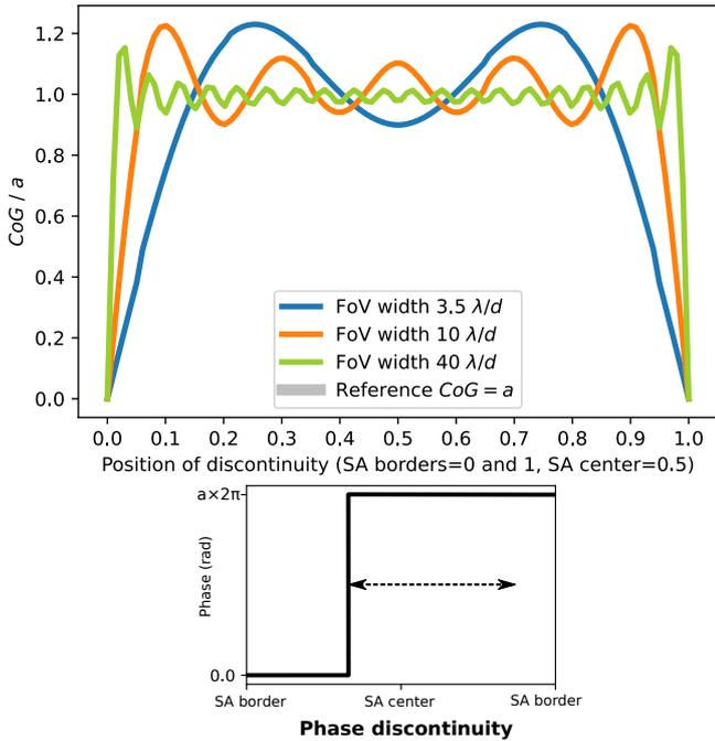
**Fig. 1.** Impact of the position of the phase discontinuity on the CoG measurement. *Top*: sensitivity to a phase discontinuity with respect to the position of the discontinuity in the subaperture (SA) for different fields of view (FoV). The simulation is carried out for  $a = 0.05$  (weak-phase regime). *Bottom*: 1D illustration of the free parameter, the position of the discontinuity.
