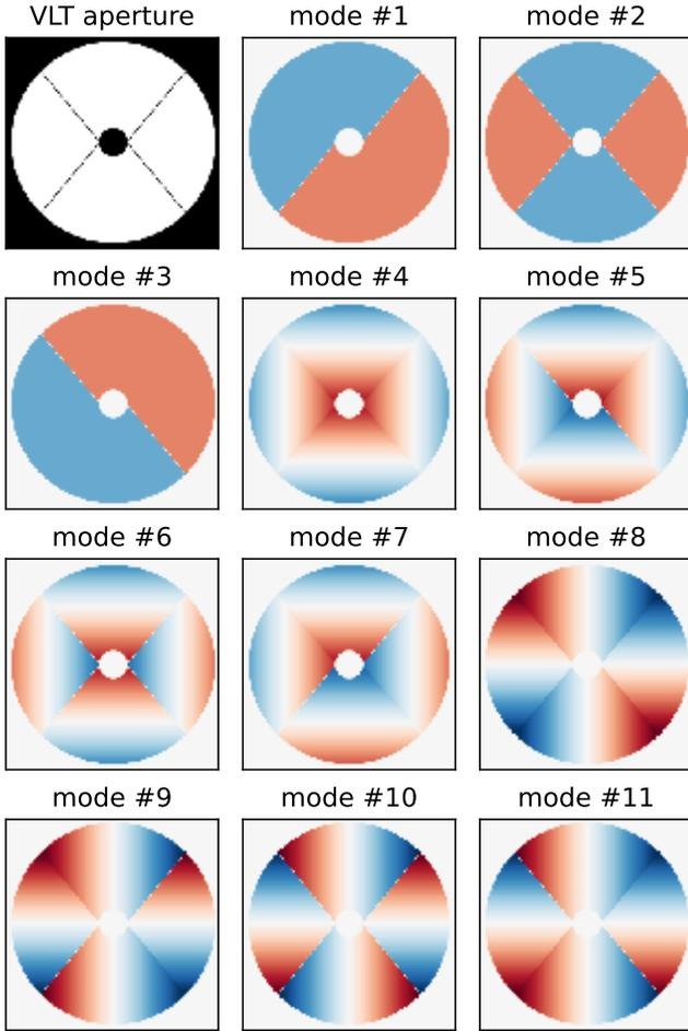
**Fig. 8.** 11 orthogonal LWE modes of the VLT pupil used in this study as pupil-plane perturbations. This compares to the classical decomposition shown in Fig. 6 of Sauvage et al. (2016a). Modes #1 to #3 are PP modes. Modes #4 to #11 are PTT modes. Odd numbers are for odd modes and even numbers are for even modes. Modes #4 and #8 do not contain discontinuities, and are removed from the control basis. Mode #10 controls the global curl pattern seen in Fig. 5.
