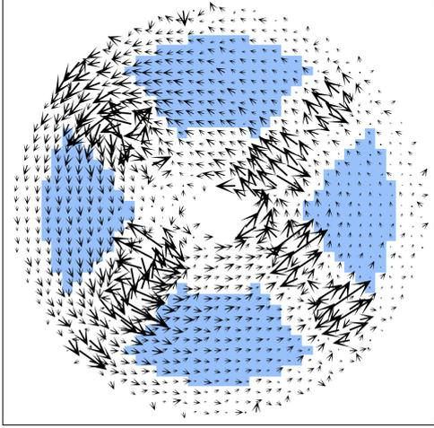
**Fig. 9.** SH slope map. The blue region highlights the subapertures that are used to estimate the PTT modes. Subapertures located close to the spiders, the secondary mirror, and the outer pupil ring are discarded.
