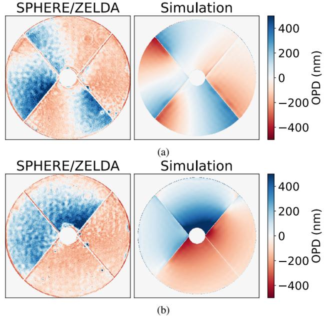
**Fig. 7.** Qualitative comparison between ZELDA measurements (*left*) and simulated post-AO residuals (*right*) for two LWE events (*a*) and (*b*). The ZELDA measurements have a 1 second detector integration time. They were taken during the night of 2014 October 8. The simulations match the typical SPHERE configuration. The result after convergence of the loop is shown here.
