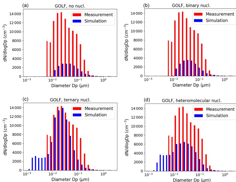
**Figure 9.** Size distribution of the number concentrations (in  $\text{cm}^{-3}$ ) at the GOLF site for the simulation without nucleation (a), with binary nucleation (b), with ternary nucleation (c), and with heteromolecular nucleation (d).
