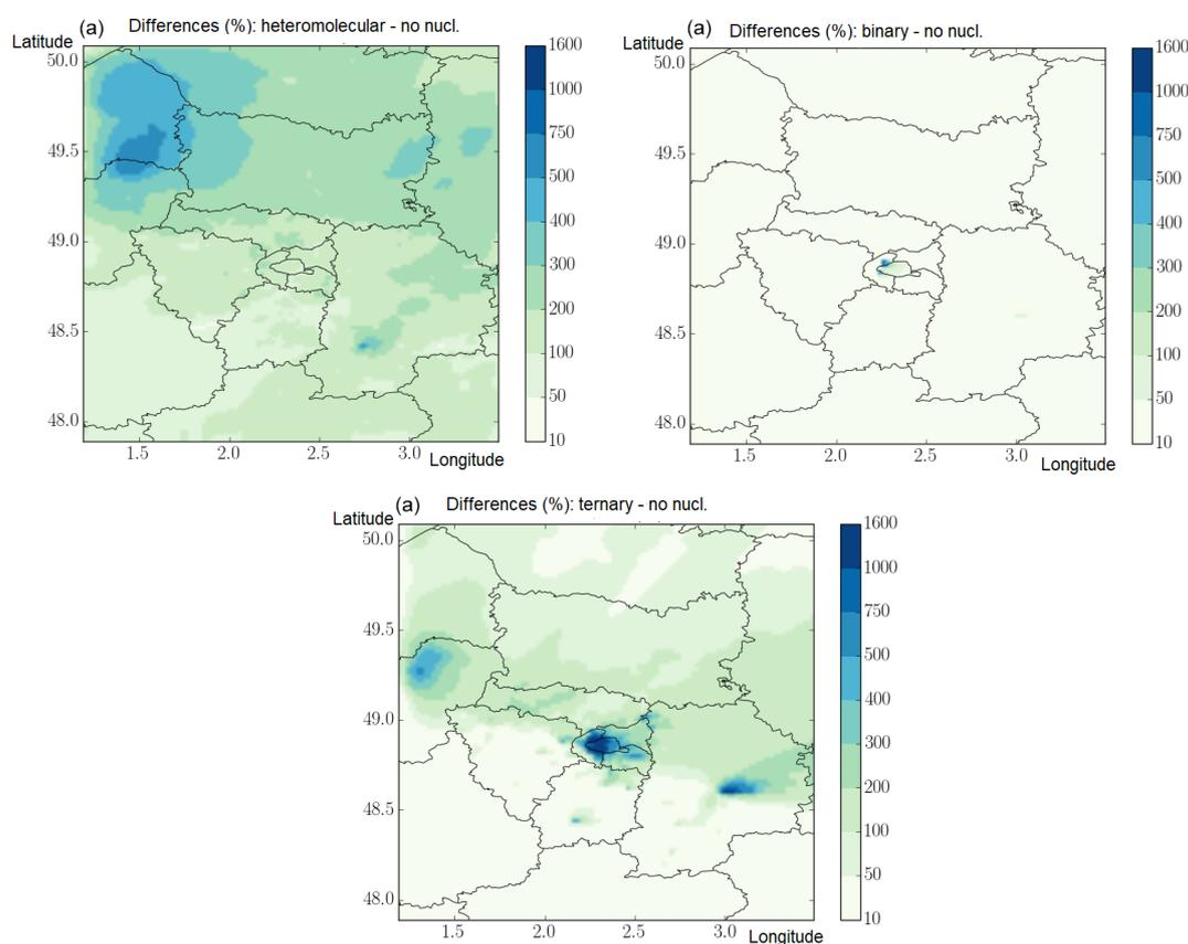
**Figure 5.** Differences in number concentrations (in %) between simulations with and without nucleation. The nucleation parameterisations used are the heteromolecular (a), the binary (b), and the ternary (c).
