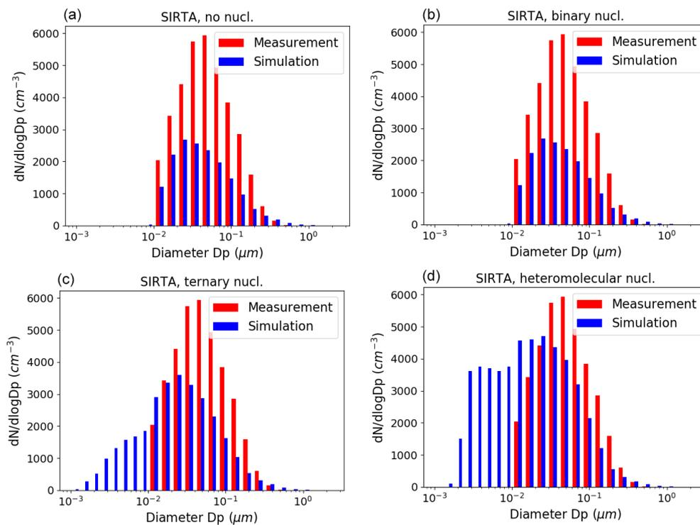
**Figure 7.** Size distribution of the number concentrations (in  $\text{cm}^{-3}$ ) at the SIRTa site for the simulation without nucleation (a), with binary nucleation (b), with ternary nucleation (c), and with heteromolecular nucleation (d).
