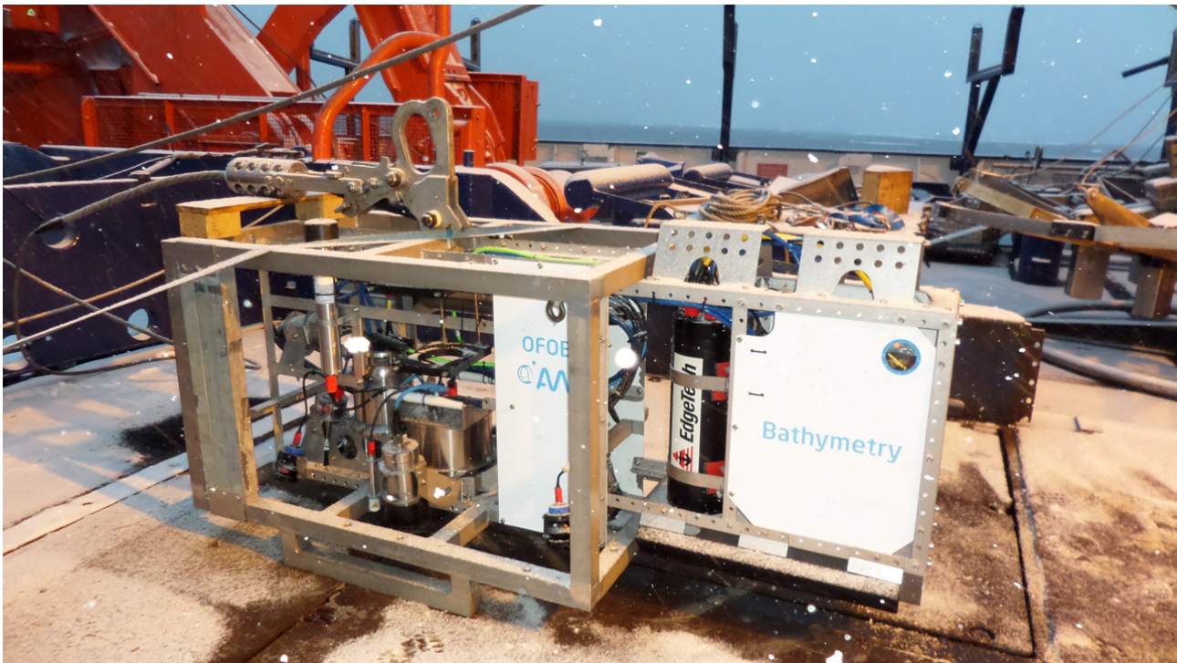
Figure 1. The Ocean Floor Observation and Bathymetry System (OFOBS) of the Alfred Wegener Institute (AWI), Helmholtz Centre for Polar and Marine Research, on deck awaiting deployment during the PS124 expedition to the southern Weddell Sea (February–March 2021).
