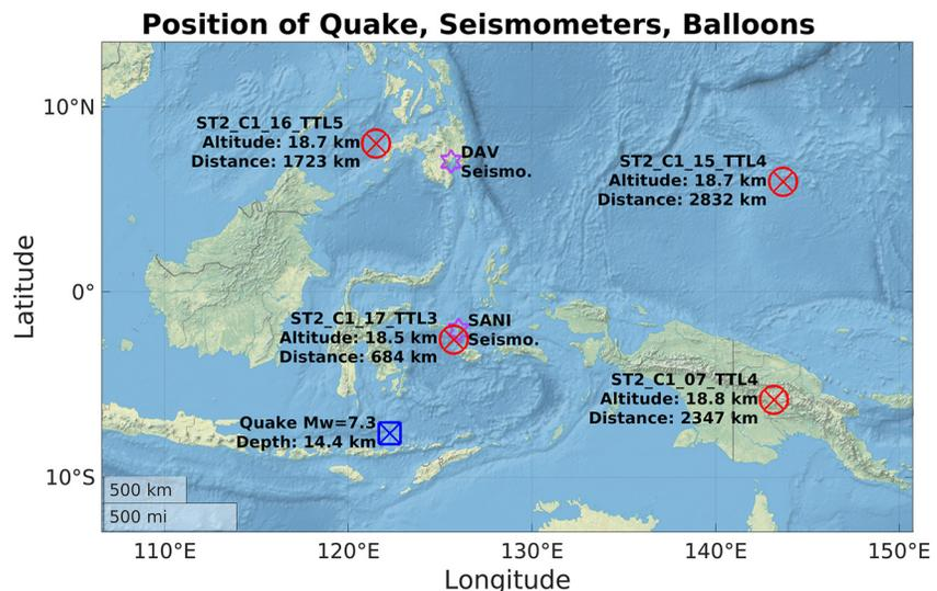
**Figure 1.** Position of the quake in Flores Sea (Blue square), the ground seismometers (purple stars) and Strateole-2 balloons (red circles) during the event. Balloon names, altitude and horizontal distance to the quake are also provided.
