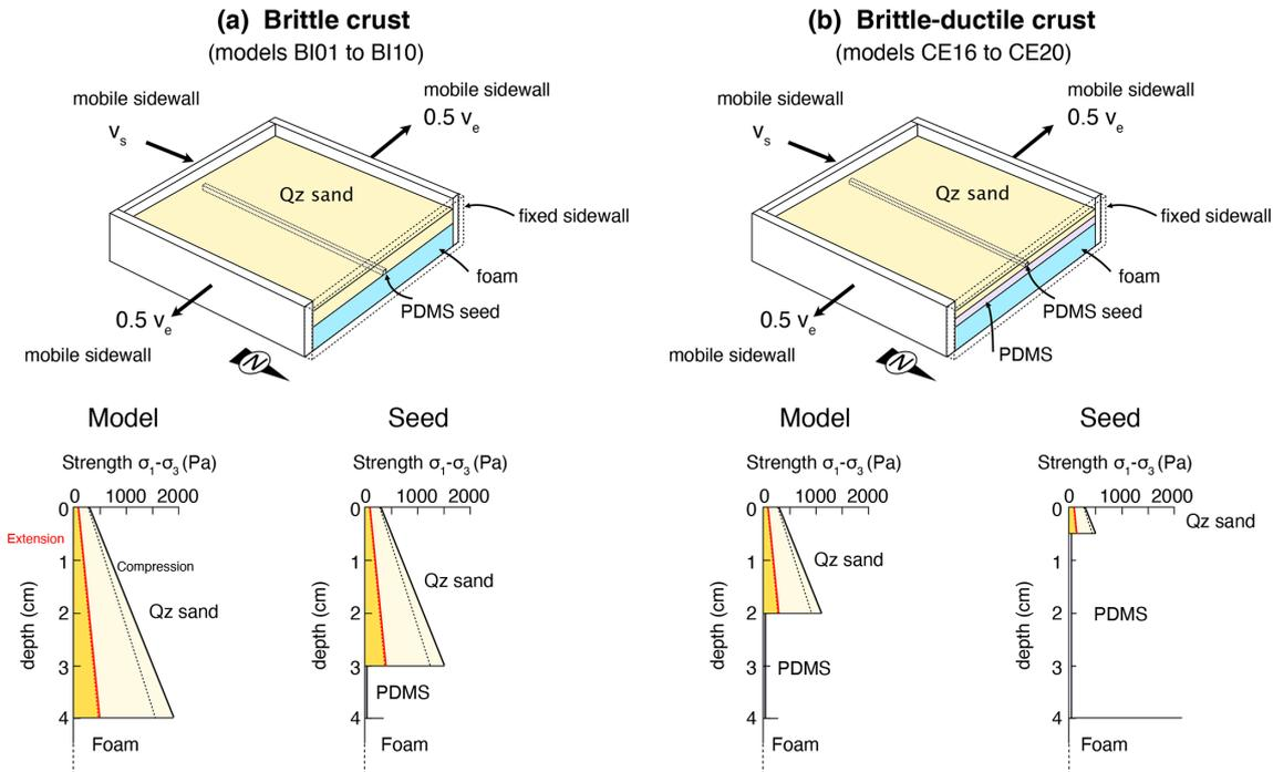
**Figure 2.** Experimental setup (top) and corresponding strength envelopes (bottom) under extension and compression for (a) models with brittle crust (“strong” crust) and (b) models with a brittle–ductile crust (“weak” crust). Solid lines correspond to the peak friction for Qz sand and dashed lines to the reactivation friction.
