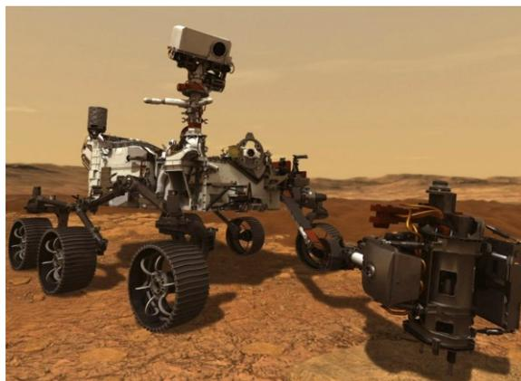
**Figure 1.** Artist's concept of the Perseverance Rover on the surface of Mars. MEDA has sensors on the mast and on the rover itself (see also Fig. 2). The Humidity Sensor (HS) is near the one of the Wind Sensor (WS) booms on the mast and also near some of the Atmospheric Temperature Sensors (ATS). Image credit: NASA
