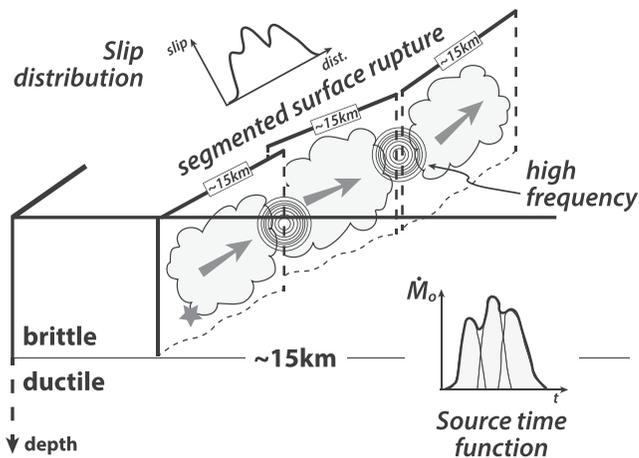
**Figure 1.** Schematic view of a strike-slip rupture including 3 sub-events. Interactions between nearby fault segments with different azimuth are generating additional high-frequencies. Independent evidence of consistent segmentation scaling are also found in surface-slip distribution, kinematic inversion results, source time function, and surface rupture geometry.
