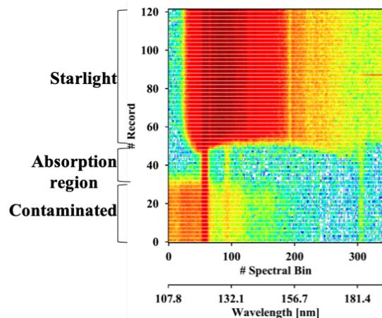
Figure 1. An example of a dayside FUV spectrum with the unattenuated stellar spectrum, rescuable finite absorption region, and stray light contaminated records.
