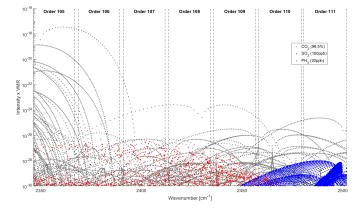
**Fig. 1.** Position of the  $CO_2$  (gray),  $PH_3$  (red), and  $SO_2$  (blue) rovibrational transitions in the 2348 to 2501 cm<sup>-1</sup> region, corresponding to the SOIR 105 to 111 diffraction orders from HITRAN (Gordon et al. 2017). The line intensities were multiplied by typical Venus abundances, see legend. The SOIR orders are given at the top, with the vertical dashed lines showing their wavenumber extensions.
