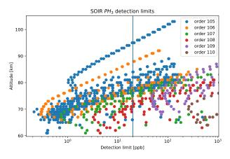
**Fig. 4.** Detection limits as a function of altitude. Colors are the different diffraction orders of SOIR. The blue vertical line corresponds to 20 ppb. The spectral range of the diffraction orders are provided in Table 1.
