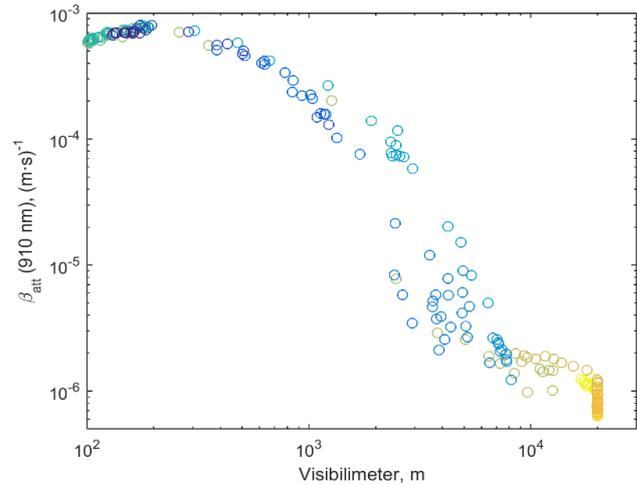
**Figure 5.** Scatter plot of simultaneous and collocated CL31  $\beta_{att}$  (905 nm) and diffusiometer visibility (550 nm) measured at 20 m a.g.l.
