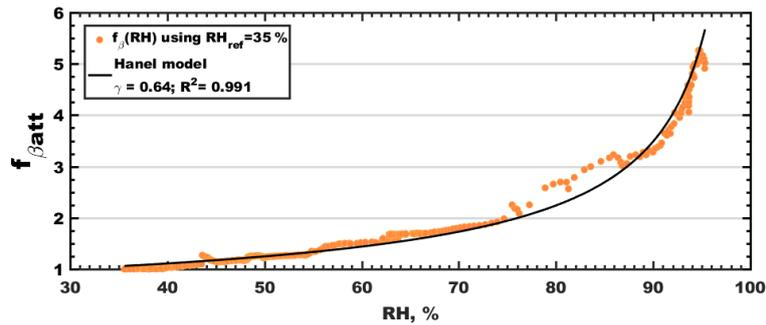
**Figure 3.**  $f_{\beta_{\text{att}}}(\text{RH})$  as function of relative humidity (orange dots) measured at 30 m a.g.l. on 10 March 2013 at SIRT and its Hänel function fit (black line).
