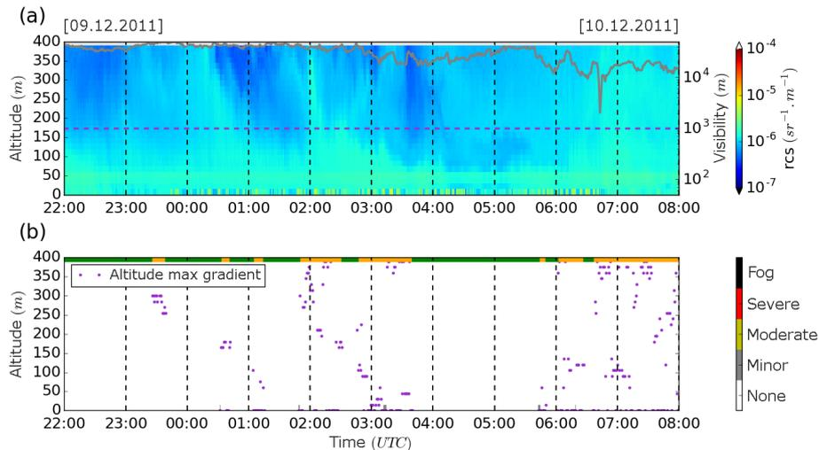
**Figure 9.** Time series presenting measurements and alert levels in pre-fog conditions on 9–10 December 2011 at SIRTA. **(a)** ALC-attenuated backscatter (color contours) and horizontal visibility (gray line) measured at 3 m a.g.l. **(b)** Alert levels (colors) and altitude of  $H_{\text{max}}$ . Pre-fog conditions are cloud-free.
