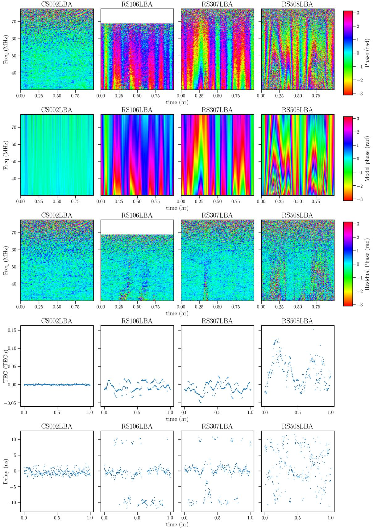
**Fig. 3.** Example direction-independent phase solutions on the target field, taken from the fourth hour of observation L667924. From top to bottom the panels show the raw phase solutions, the TEC+Delay model phases, the phase residuals, and the fitted TEC and Delay terms as a function of time.
