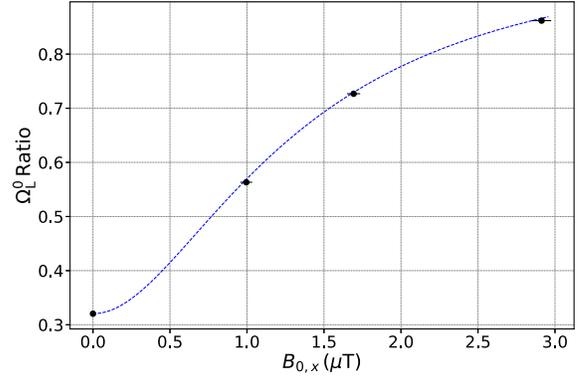
FIG. 1.  $B_{0x}$  calibration data obtained for the dressed  $B_t = 0$  case at  $\omega_{0z}/2\pi = 5.979(2)$  kHz and  $\omega/2\pi = 30$  kHz. The ratio of the  $\Omega_L^0$  measurements at the  $\xi = 0$  and  $\xi = 1.833(5)$  values vs  $B_{0x}$  is marked by the black dots. The fit to the theoretical predictions determines the  $B_{0x}$  scale at the four percent precision level given by the horizontal error bars. The  $B_{0x} = 0$  data point provides the  $\xi$  calibration.
