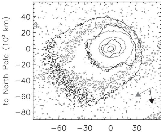
**Figure 9.** Isophotes of the observed (grey isophotes) and of the model (black isophotes) dust tail of comet C/2020F2 at  $r_h = 9.17$  au. Black arrow: antisolar direction. Grey arrow: trailing orbit direction. The tail model assumes no dust ejection from nucleus latitudes  $< -60$  and  $> +60$  deg, with a lower  $d = 0.122$ .
