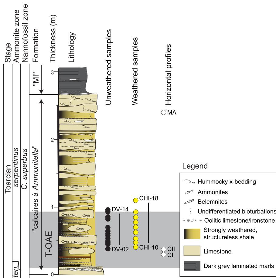
**Figure 2.** Lithological succession of the Lafarge cement quarry (modified after Suan et al., 2003). The biostratigraphic zonation is based on ammonites and calcareous nannofossils (Suan et al., 2013). Stratigraphic position of the weathered and unweathered bulk rock samples and horizontal profiles are shown.
