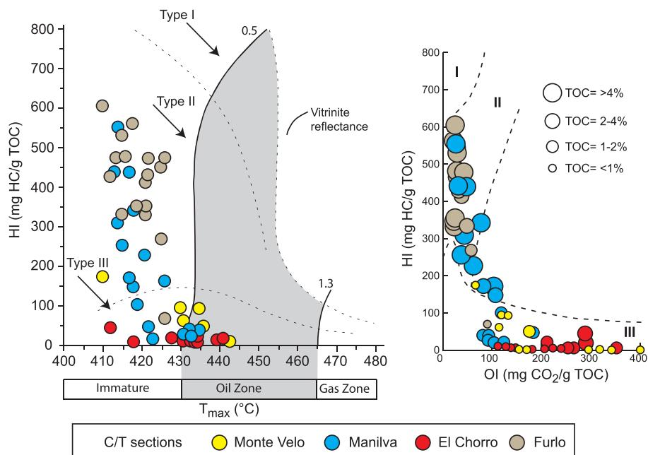
**Figure 9.** HI/ $T_{\text{max}}$  diagram for preserved organic matter (OM) and cross plot between Oxygen Index (OI, mg CO<sub>2</sub>/g TOC) and Hydrogen Index (HI, mg HC/g TOC) for Furlo, Manilva, Monte Velo, and El Chorro sections in a modified van Krevelen-type diagram, showing the different types of organic matter (Espitalié et al., 1985).
