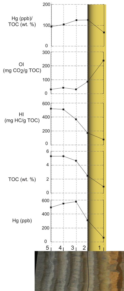
**Figure 6.** Hg (ppb), TOC (wt.%), HI (mg HC/g TOC), OI (mg CO<sub>2</sub>/g TOC), and Hg/TOC (ppb/wt.%) ratios along horizontal profile MA (*H. bifrons* ammonite Zone). The yellow bars represent the weathered edges of the horizontal horizons.
