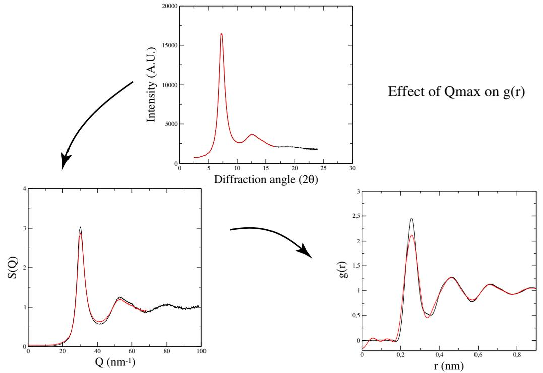
**Figure 5.** Effects on the obtained  $g(r)$  from the modification of the  $Q$  ranges to  $100 \text{ nm}^{-1}$  in black and to  $70 \text{ nm}^{-1}$  in red. The peak positions are not affected, but their respective height and width are modified.
