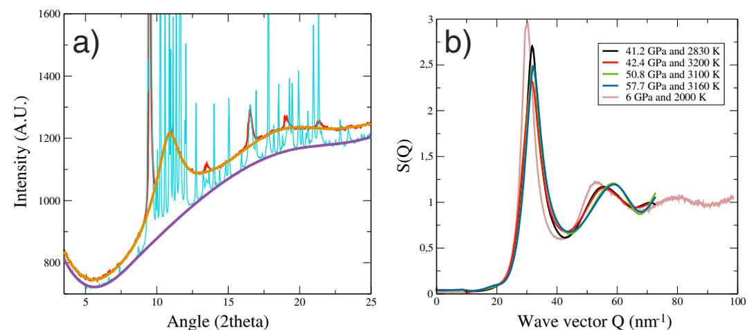
**Figure 2.** (a) Diffraction patterns before (turquoise) and after (red) melting in a LH-DAC experiment at 50.8 GPa. The diffuse scattering pattern from a liquid Fe-C alloy is shown by orange line, after subtracting spurious diffraction peaks from the pressure medium and solid phases. The background (purple line) was acquired from an X-ray diffraction pattern (turquoise line) before melting. (b) Structure factors  $S(Q)$  of the liquids studied here at different *P-T* conditions.
