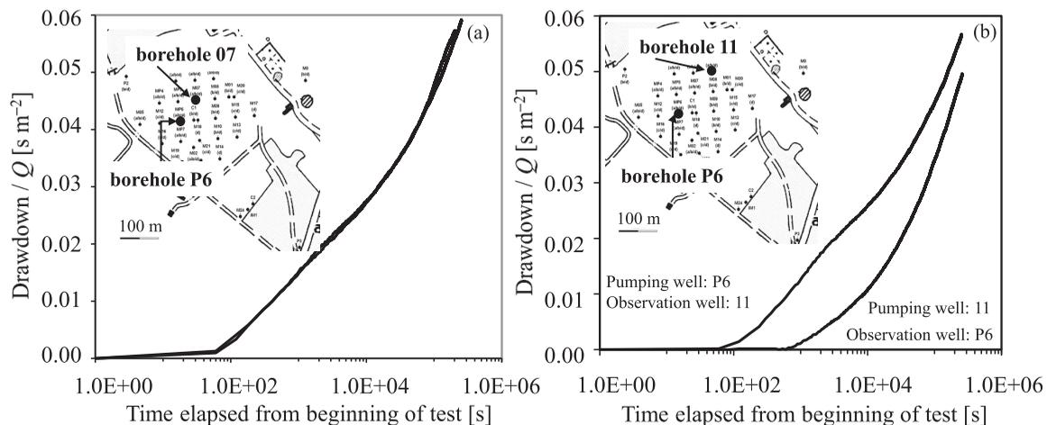
**Figure 1.** Drawdown curves observed during interference pumping tests performed at the Hydrogeological Experimental Site (HES): (a) example of reciprocity detected between wells P6 and 07; (b) example of observed reciprocity gaps between wells P6 and 11. Figure adapted from Delay *et al.* [2011].
