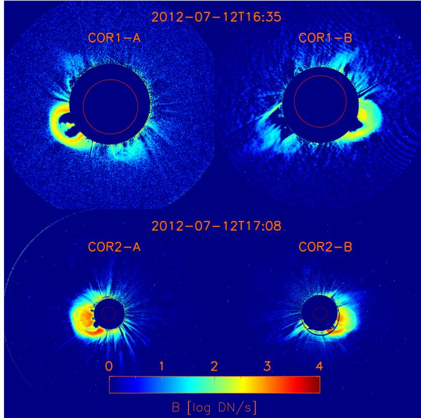
**Figure 4.** Total brightness from COR1-A (*upper-left panel*), COR1-B (*upper-right panel*), COR2-A (*lower-left panel*) and COR2-B (*lower-right panel*) observations. The images are displayed in logarithmic scale. Base-difference images were used. The circle inside the occulter outlines the solar disk.
