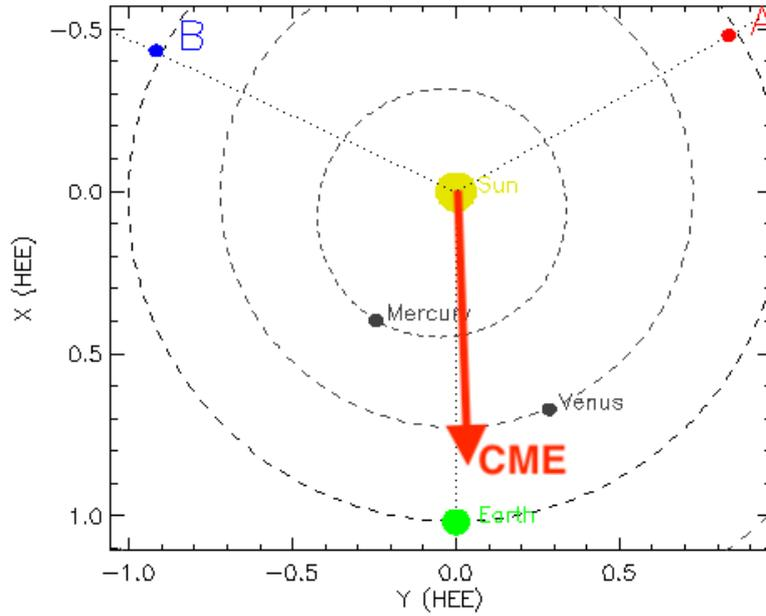
**Figure 10.** Position of the three spacecraft (STEREO-A (*red*), STEREO-B (*blue*), and SOHO - Earth perspective (*green*) on 12 July 2012, 16:00). The red arrow indicates the direction of propagation of the CME as derived from GCS reconstruction. The view is from above, in the Heliocentric Earth Ecliptic (HEE) coordinate system, with  $x$ -axis towards the Earth and its  $z$ -axis towards Ecliptic North Pole (Thompson, 2006).
