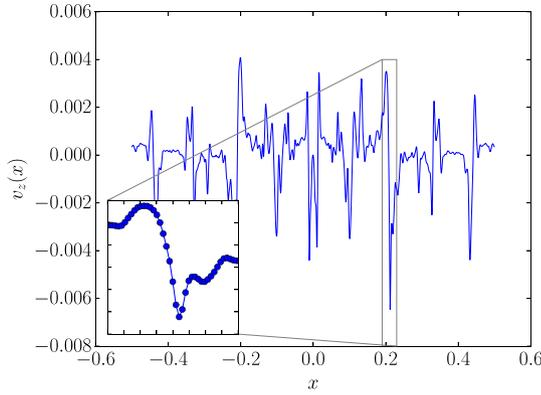
**Figure 3.** Vertical velocity as a function of  $x$  measured at  $z = 0.1$  in run v7-1024-v at  $t = 600$ . The inset zooms on the critical layer at  $x \simeq 0.21$  with dots representing the spectral collocation points. Note the sharpness of the critical layers despite the large resolution.
