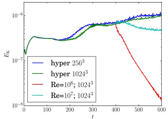
**Figure 2.** Volume averaged kinetic energy as a function of time for several simulations at  $\text{Fr} = 2$  and  $q = 3/2$ . The blue curve corresponds to our fiducial case. High-resolution runs including diffusion are restarted from the hyperdiffusion run at  $t = 400$ .
