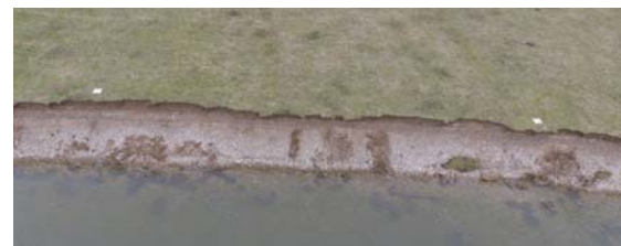
Figure 3: Bank morphology and coded targets as GCPs
