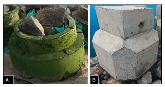
**Figure 1**. A: Accroberm<sup>TM</sup> II (2.24 m diameter); B: 'double cube' unit (1.3 m nominal diameter)
