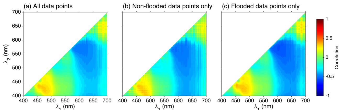
**Figure 5.** Correlation surfaces of normalized difference indices (NDI) for snow depth for (a) all data points, (b) nonflooded data points only, and (c) flooded data points only.  $\lambda_1$  and  $\lambda_2$  indicate the used wavelength pairs according to equation (4).
