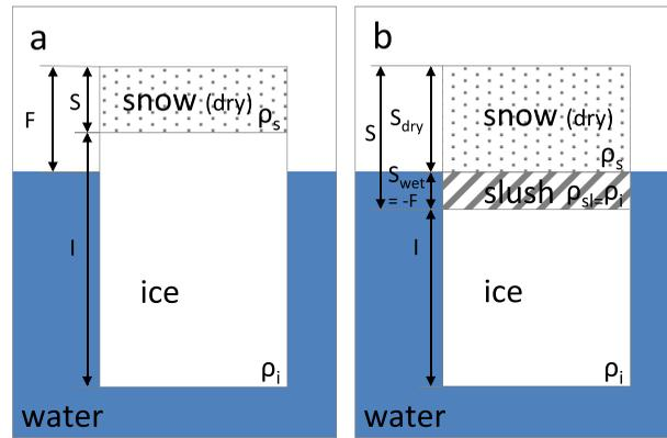
**Figure 2.** Two typical states of Antarctic sea ice. (a) Positive freeboard with the snow/ice interface above the sea level. (b) Negative freeboard with the snow/ice interface below the sea level. The flooded snow (slush) is referred to as (negative) freeboard and is assumed to have the same density as sea ice.
