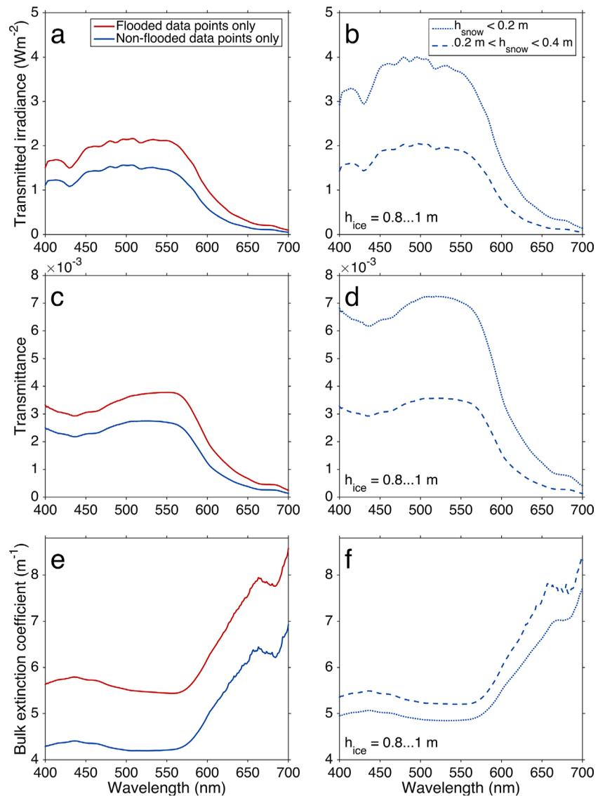
**Figure 6.** Mean spectral (a and b) transmitted irradiance, (c and d) light transmittance, and (e and f) bulk extinction coefficient for (a, c, e) flooded data points only (red), nonflooded data points only (blue) and (b, d, f) nonflooded data points only with a sea-ice thickness between 0.8 and 1 m subdivided into two snow classes: snow depth  $< 0.2$  m (dotted lines) and snow depth  $> 0.2$  m and  $< 0.4$  m (dashed lines).
