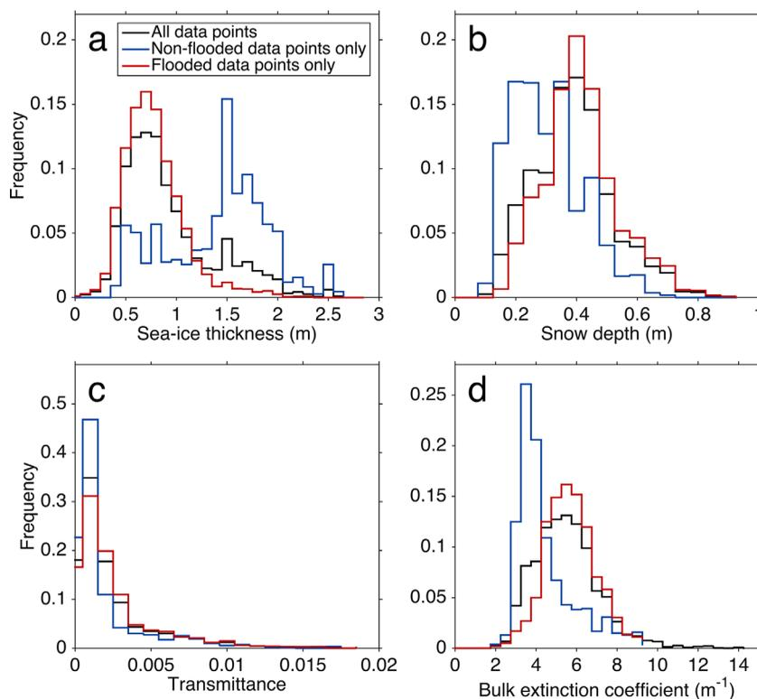
**Figure 4.** Histograms of (a) sea-ice thickness, (b) snow depth, (c) light transmittance, and (d) calculated bulk light extinction coefficients for the entire data set (black), nonflooded data points only (blue), and flooded data points only (red).
