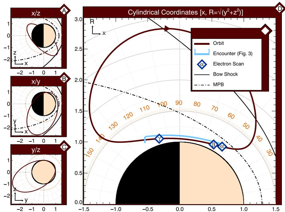
**Figure 3.** Map of MAVEN orbit № 867. The coordinate system is Mars Solar Orbital (MSO), where x points toward the Sun, y points backward along the tangent of the planetary orbit, and z completes the right-handed set pointing up out of the plane of the ecliptic out of the northern hemisphere. The orbit of the MAVEN Mars Scout is shown in maroon, with a model bow shock and magnetic pileup boundary (ionopause) in black, according to Vignes et al. [2000].
