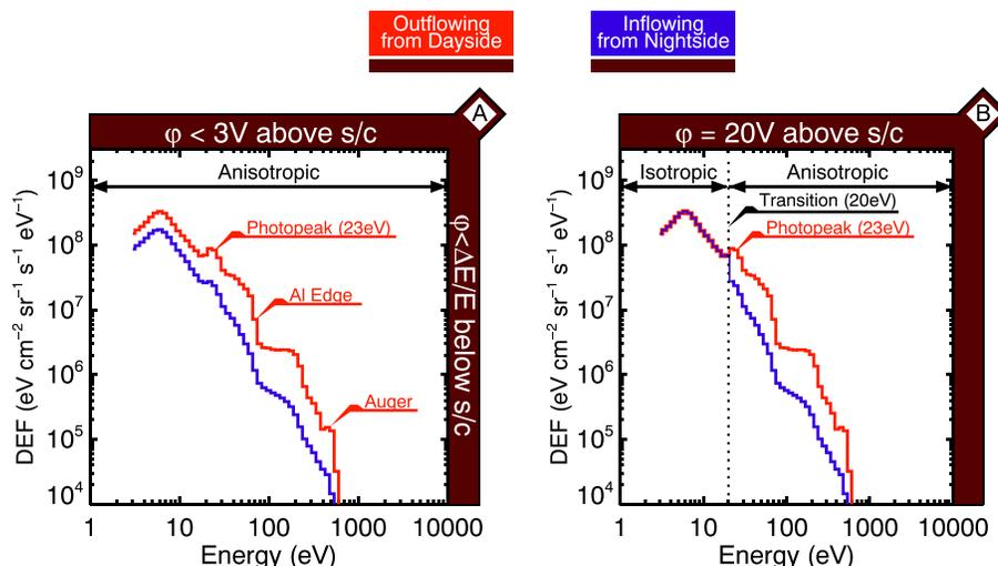
**Figure 2.** Sketches showing the predicted spectra of photoelectrons in the tail of Mars for two hypothetical electric potential drops: (a) Electric potential drop  $\phi < 3$  V above MAVEN; (b) Electric potential drop  $\phi = 20$  V above MAVEN. The predicted spectra of electrons flowing outward from the dayside source region are shown in red and the hypothetical spectra of electrons flowing back from the nightside in blue.
