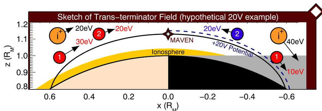
**Figure 1.** Schematic of a hypothetical trans-terminator magnetic field line, with 20 V electric potential drop on the nightside, and its effect on three particles; electron N° 1, born with an energy of 30 eV and impacting the nightside ionosphere; electron N° 2, born with an energy of 20 eV and being reflected back to the dayside; and an ion ( $i^+$ ) born with an energy of 20 eV and accelerated by the potential drop into the nightside ionosphere.
