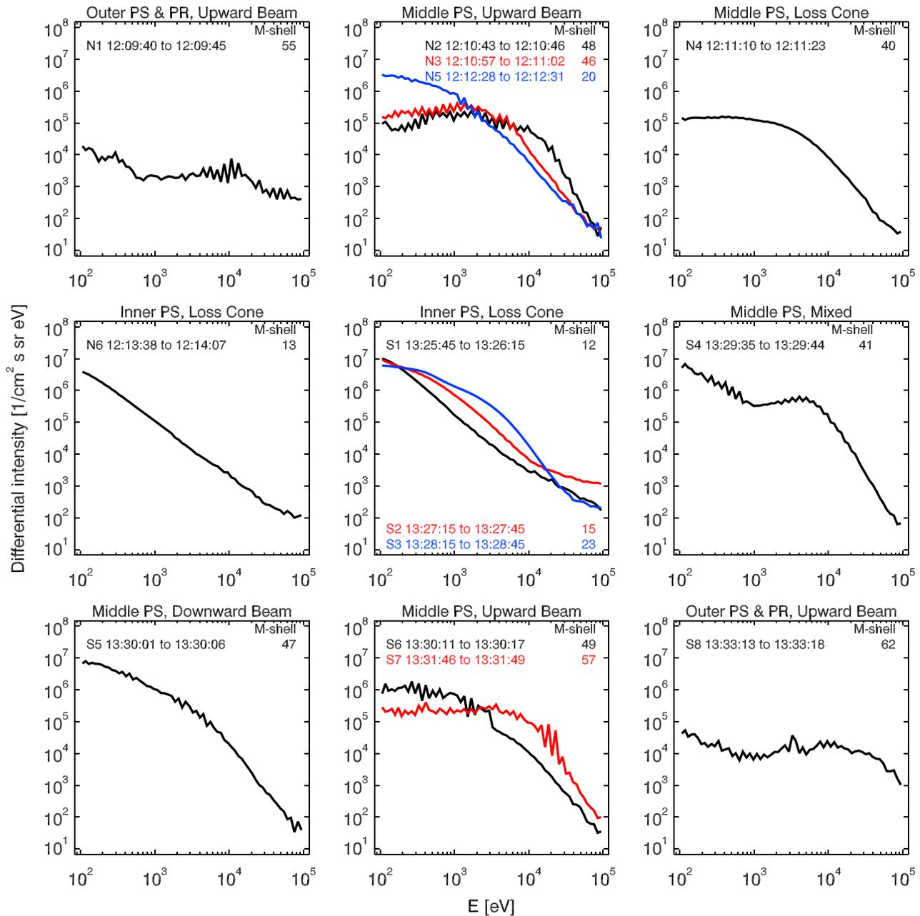
**Figure 4.** Electron differential intensities (averaged over look directions) as functions of energy for the intervals indicated with the black bars on top of Figures 1c and 2c. The corresponding region is indicated in the title of each panel, and the interval label and time ranges are given in the plots.
