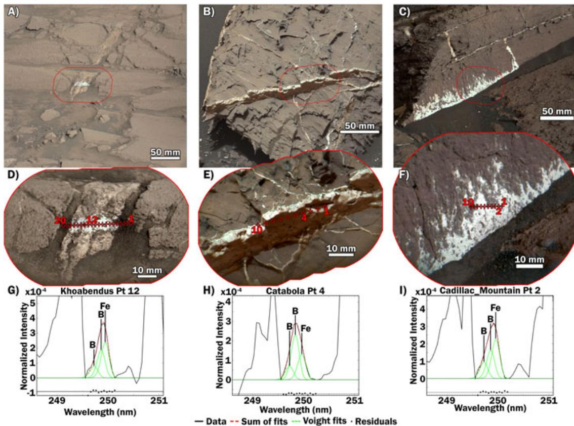
**Figure 1.** Three examples of boron detections in Murray unit vein targets. (a–c) Mastcam context images with RMI footprints (red outlines), (d–f) colorized RMIs labeled with point observations (numbered crosshairs), and (g–i) example LIBS spectra with boron and iron line fits for “Khoabendus” (sol 1380), “Catabola” (sol 1443), and “Cadillac\_Mountain” (sol 1504) (Mastcam images 1381MR0067690000701773E01, 1444MR0071420000702955E01, and 1504MR0076390000404439E01).
