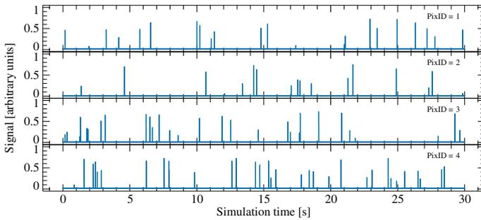
**Fig. 3** Individual signals of a four-pixel configuration during a 30 s simulation with random photon impacts. The currents are flipped and normalized to the range 0–1 (Color figure online)
