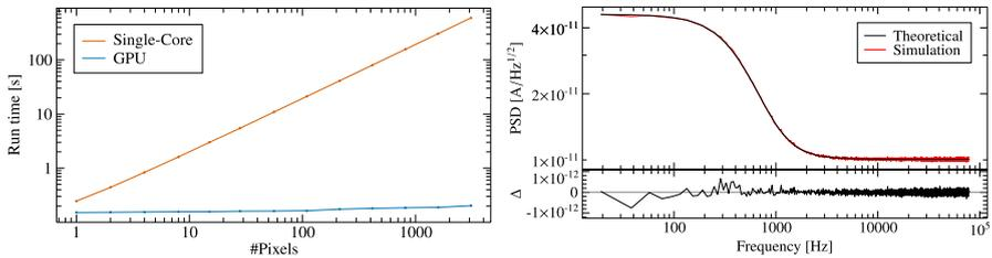
**Fig. 4** Left: Run time comparison between single-core and GPU-accelerated version of our code (using single-precision arithmetic on an Nvidia GeForce GTX 1080 Ti GPU) for different array sizes simulated for 1 s each. Right: Comparison between predicted and simulated noise levels. The bottom panel shows the differences between the two results (Color figure online)
