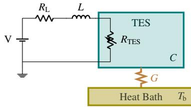
**Fig. 2** Diagram of the electrothermal system that we implement in our software, consisting of the Thevenin-equivalent representation of the bias circuit coupled to the TES (after [1]). An equivalent bias voltage  $V$  is applied to a load resistor  $R_L$ , an inductance  $L$ , and the TES. We assume the TES to have a heat capacity  $C$ , which is connected to a heat bath at temperature  $T_b$  through a weak thermal link with thermal conductance  $G$  (Color figure online)
