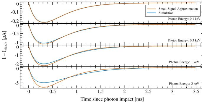
**Fig. 5** Pulse shape comparison between simulation and TES small-signal model for different photon energies. The pulses match very well for small energies. For higher energies, they start to deviate as expected due to the nonlinearity of the readout circuit (Color figure online)
