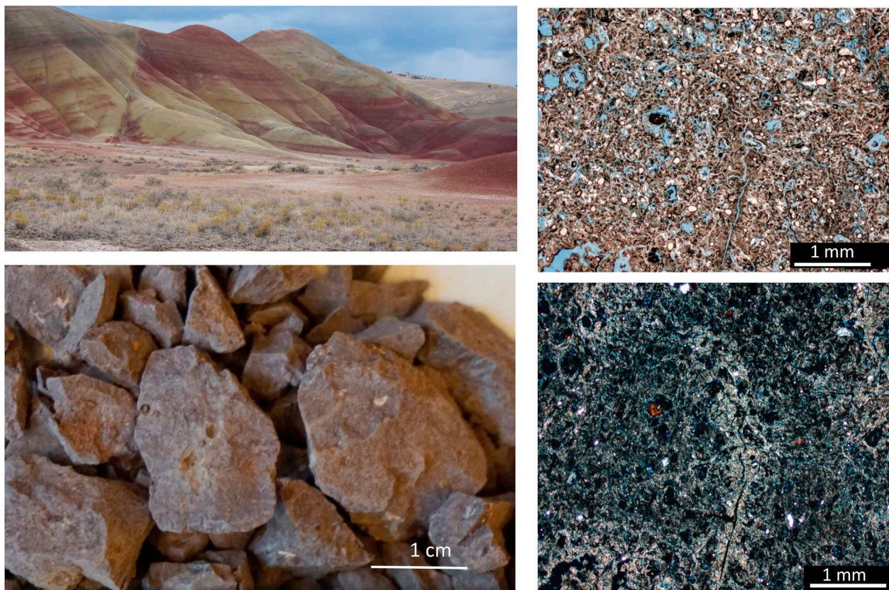
Fig. 19. Weathered tuffs, rhyolite from John Day Valley in the upper left photo. Sample JD 16–0018 (lower left) and to the right thin section photos with blue stained epoxy; upper right photo ordinary light, lower right photo crossed polarizers. Scale bar in photos.
