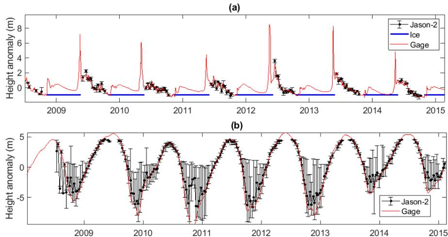
**Figure 2.** Example time series for the Mackenzie River. Panel (a) shows water surface heights with ice filtering compared to the Environment Canada gage (10KA001) located 684 km away from the virtual station. Panel (b) compares the time series derived from Jason-2 for one of the Amazon gages. Error bars represent the range of the values that were averaged to generate each data point (does not include filtered data points).
