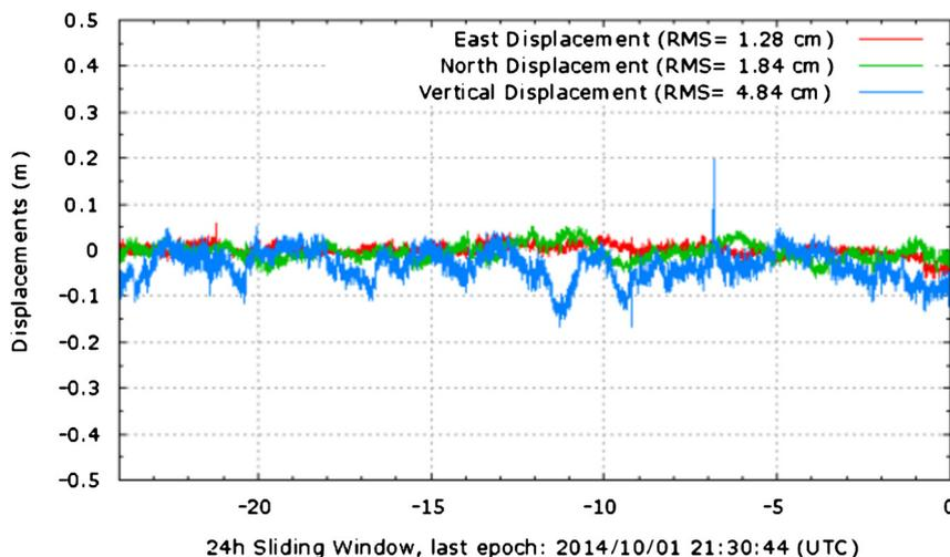
Fig. 2. Real-time (static) rover coordinate determination (<http://www.ppp-wizard.net>).
