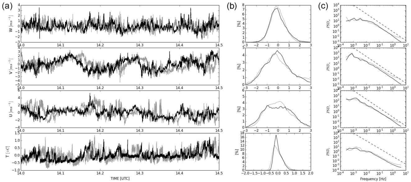
**Figure 4.** Comparison of  $w'$ ,  $v'$ ,  $u'$  and  $t'$  measured by a tethered-balloon probe (black) and a sonic anemometer (grey) fixed onto a tower nearby for (a) 10 Hz time series for 30 min, (b) fluctuation distribution of a 2 h sample, and (c) power spectra density corresponding to the same sample.
