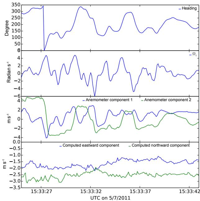
**Figure 2.** Time series of sensor orientation and wind during 20 s of a flight in the BLLAST campaign (5 July 2011). Panel's content, from top to bottom, is as follows: (top) heading – angle between the north and the first horizontal axis of the MTi-G; (upper middle) rotation rate along the  $z$  axis of the MTi-G; (lower middle) two components of the wind measured by the WindMaster anemometer along its  $x$  and  $y$  axis; and (bottom) northward and eastward components of the computed wind.
