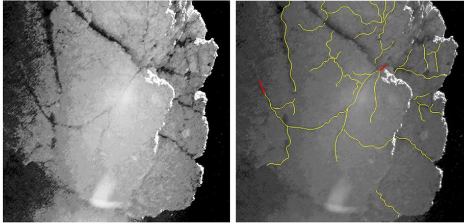
**Figure 2.** Close-up from CIVA no. 1 showing the fractured block. The left image was stretched to emphasize the fractures. The two reds arrow indicate the limit of the fracture having the maximum length (537.6 mm at  $1 \text{ mm pix}^{-1}$  resolution or 752.6 mm at  $1.4 \text{ mm pix}^{-1}$  resolution).
