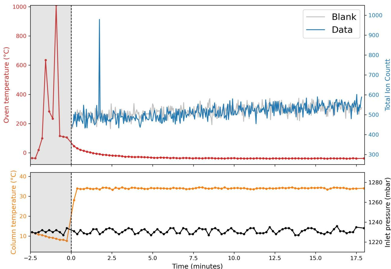
**Figure 1.** Monitoring of different relevant housekeeping parameters: oven temperature (top, red), column temperature (bottom, orange) and inlet pressure (bottom, black). On the top plot, the total ion count from the FSS mass spectra (Data) over time is shown in blue while in light grey we show the mass spectra from the gas chromatogram taken during PHC (Blank) under the same conditions. The data "peak" at around 2 minutes is a noise spike and should be disregarded.
