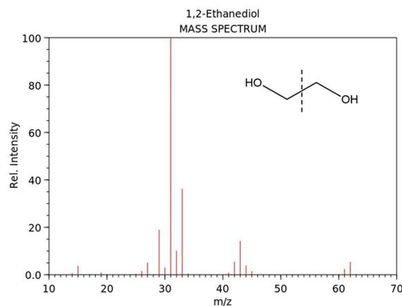
**Figure 6.** Electron Ionization (EI) mass spectrum of 1,2-ethanediol or ethylene glycol ( $C_2H_4O_2$ ). The base peak is at  $m/z$  31 and is significantly stronger than any other  $m/z$  as it represents the perfectly symmetric breaking of the molecule (shown on the top right corner), leaving 2 hydroxymethyl radicals of which either one can keep the positive charge induced by the electron impact. From NIST Chemistry WebBook (<https://webbook.nist.gov/chemistry>).
