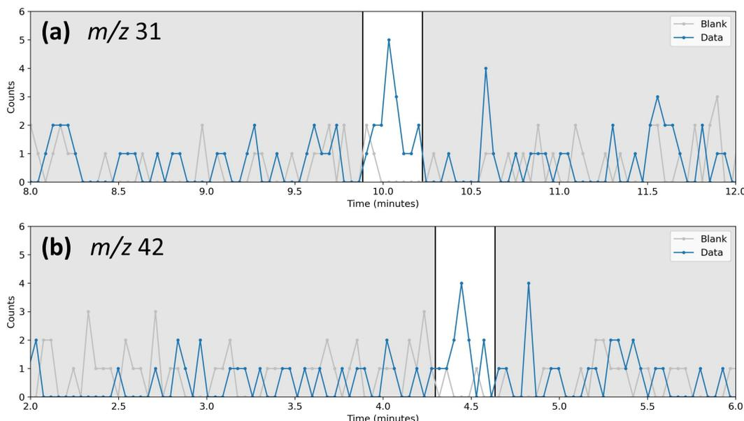
**Figure 4.** Visualization of the scanning process and of the 2 different peaks that were flagged by our algorithm. (a)  $m/z$  31: the FSS (Data) shows 17 counts against 3 in the PHC (Blank) in the highlighted time window. (b)  $m/z$  42: likewise, the FSS shows 12 counts against 2 PHC count.
