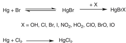
**Fig. 1** Current understanding of the formation of oxidized Hg(II) compounds from atmospheric gaseous elemental mercury initiated by different oxidant species. This figure also includes other secondary oxidation mechanisms involving single-step reactions with Cl<sub>2</sub>, O<sub>3</sub>, BrO, and ClO
