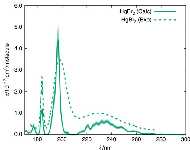
**Fig. 3** Calculated and experimental cross section of gas-phase  $\text{HgBr}_2$ . The calculated spectrum was obtained with the CASSCF/MS-CASPT2/SO RASSI methodological approach using the ANO-RCC-VTZP basis set. The light coloured areas correspond to the numerical error of absorption cross sections due to the statistical sampling
