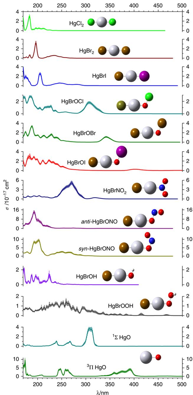
**Fig. 2** Ball-and-stick representation and computed UV-VIS absorption spectra and cross sections ( $\sigma$ ,  $\text{cm}^2$ ) of the Hg(II) compounds studied in the present work. The light-coloured areas correspond to the uncertainty of the cross section due to the statistical sampling. Note the different range of  $\sigma$  values for some of the spectra. Also note that only wavelengths  $>290$  nm are relevant for ambient tropospheric conditions
