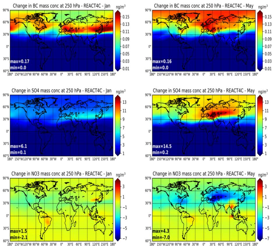
**Figure 6.** Spatial distributions of the 250 hPa perturbation due to aircraft emissions for January (left) and May (right) for BC, SO<sub>4</sub> and NO<sub>3</sub> (ng/m<sup>3</sup>) for the REACT4C\_2006 inventory.
