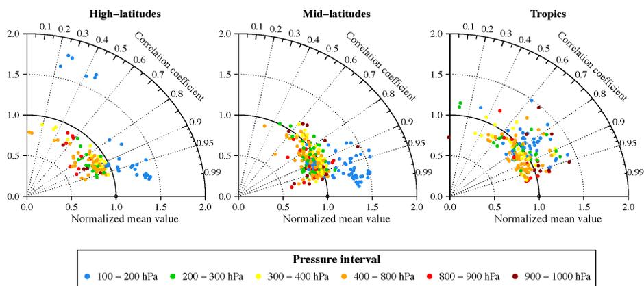
**Figure 1.** Taylor diagram comparing the mean and temporal correlation of ozone volume mixing ratio between ozonesonde climatology over the 1995-2011 period (Tilmes et al., 2012) and LMDZ-INCA model results, interpolated to the sample locations and interpolated on six pressure levels for high-latitudes, mid-latitudes and tropical stations.
