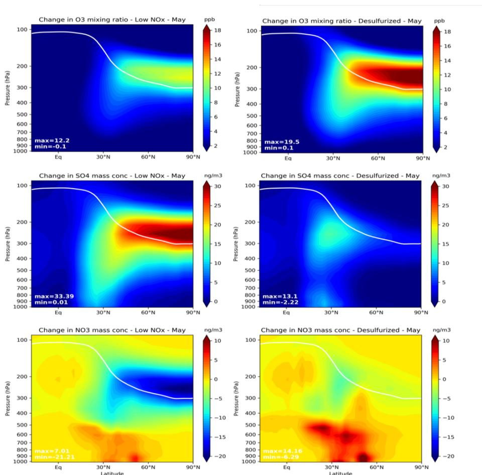
**Figure 10.** Zonal mean perturbation due to aircraft emissions for May of O<sub>3</sub> (ppbv), SO<sub>4</sub> and NO<sub>3</sub> (ng/m<sup>3</sup>) for the LowNOx (left) and Desulfurized (right) scenarios. The solid line represents the tropopause pressure.
