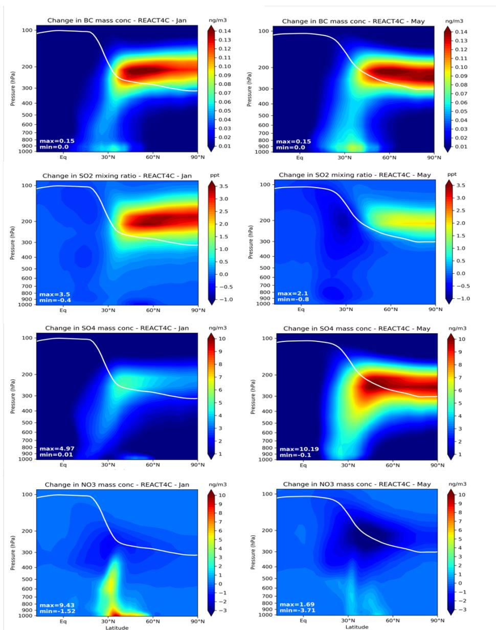
**Figure 7.** Zonal mean perturbation due to aircraft emissions for January (left) and May (right) of BC (ng/m<sup>3</sup>), SO<sub>2</sub> (pptv), SO<sub>4</sub> (ng/m<sup>3</sup>) and NO<sub>3</sub> (ng/m<sup>3</sup>) for the REACT4C\_2006 inventory. The solid line represents the tropopause pressure.
