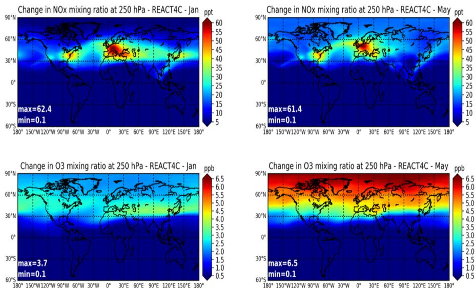
**Figure 4.** Spatial distribution of the 250 hPa perturbation due to aircraft emissions for the month of January (left) and May (right) for NOx (pptv) and ozone (ppbv) mixing ratio for the REACT4C\_2006 inventory.
