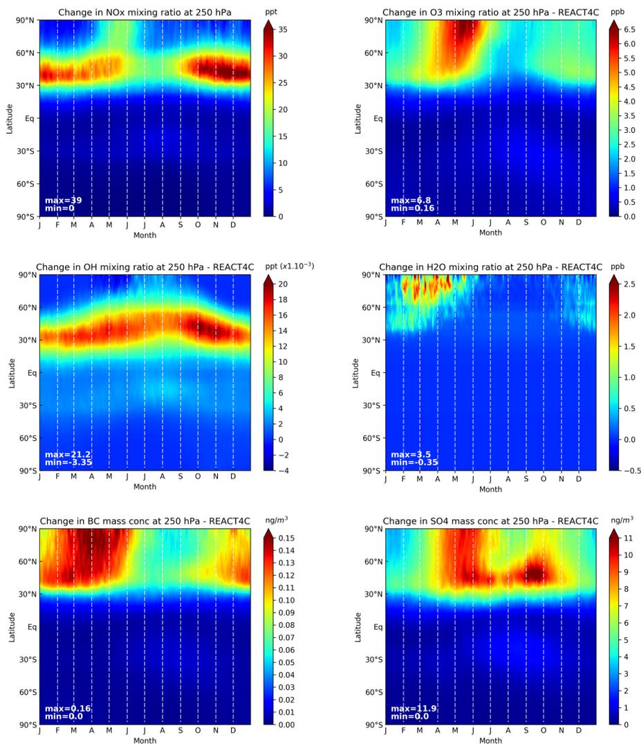
**Figure 3.** Daily and zonally averaged perturbation due to aircraft emissions at 250 hPa of NO<sub>x</sub> (pptv), O<sub>3</sub> (ppbv), OH ( $10^{-3}$  pptv), H<sub>2</sub>O (ppbv), BC (ng/m<sup>3</sup>) and SO<sub>4</sub> (ng/m<sup>3</sup>) for the REACT4C\_2006 inventory.
