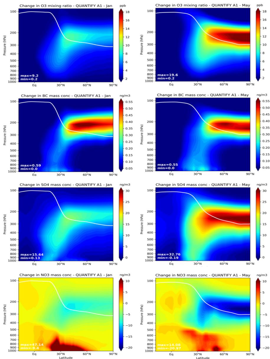
**Figure 9.** Zonal mean perturbation due to aircraft emissions for the months of January (left) and May (right) for O<sub>3</sub> (ppbv), BC (ng/m<sup>3</sup>), SO<sub>4</sub> (ng/m<sup>3</sup>) and NO<sub>3</sub> (ng/m<sup>3</sup>) averaged for the future scenario QUANTIFY A1 2050. The solid line represents the tropopause pressure.
