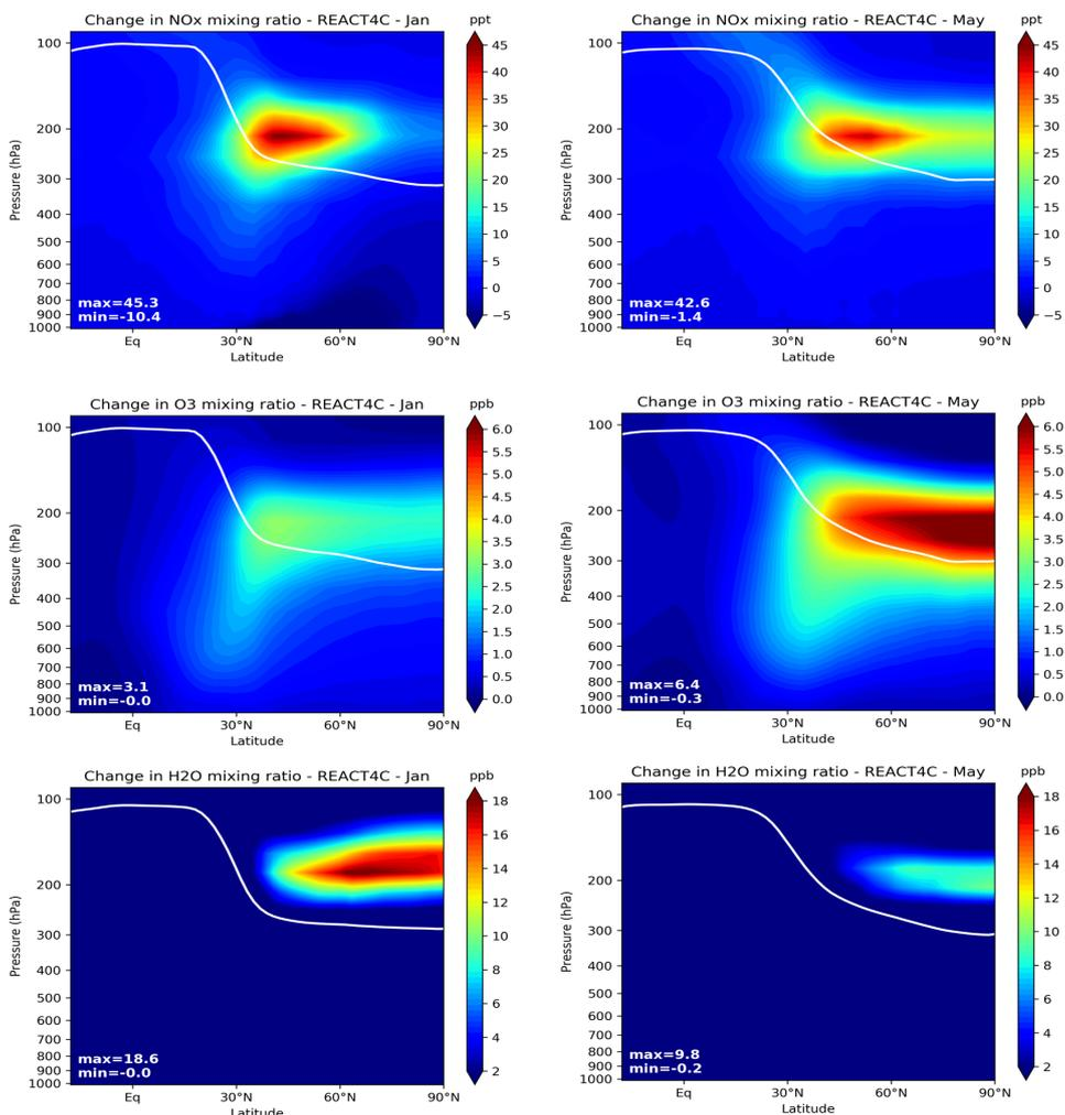
**Figure 5.** Zonal mean perturbation due to aircraft emissions for January (left) and May (right) of NO<sub>x</sub> (pptv), O<sub>3</sub> (ppbv), and H<sub>2</sub>O (ppbv) for the REACT4C\_2006 inventory. The solid line represents the model tropopause pressure.
