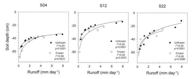
**Figure 6.** Relationships between runoff and groundwater levels along the soil transect. There was a statistically significant difference between the relationships based on data from periods with and without soil frost for all three profiles.
