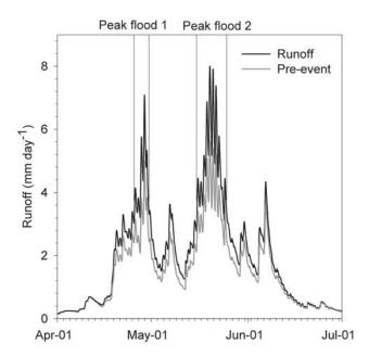
**Figure 2.** Separation of event and preevent water in Västrabäcken. "Peak flow 1" and "Peak flow 2" are marked for reference in the text.
