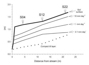
**Figure 7.** Schematic figure of the hillslope transect with groundwater levels associated with a given runoff.
