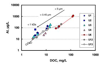
**Fig. 13.** Correlation between Al and DOC in filtrates and dialysates of various samples shown by different symbols (see Table 1 for description). In each series, the first (highest) point corresponds to filtration through 5 or  $0.45~\mu m$  and the lowest point represents dialysis through 1~kDa.
