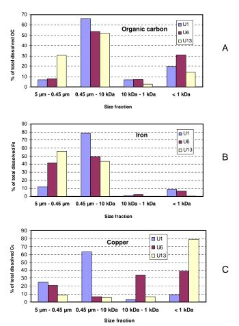
**Fig. 15.** Size fractionation of OC (**A**), Fe (**B**) and Cu (**C**) among main colloidal and subcolloidal fractions in typical samples reflecting three main stages of thaw lake development: U-6, U-1 and U-13 corresponding to peat abrasion, large growing lake and final (khasyrey stage) of the lake.
