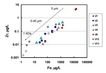
**Fig. 14.** Correlation between Zr and Fe in filtrates and dialysates of various samples shown by different symbols. In each series, the first (highest) point corresponds to filtration through 5 or 0.45  $\mu$ m and the lowest point represents dialysis through 1 kDa.
