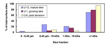
**Fig. 17.** Percentage of Fe colloids surface sites present in various size fractions for three typical stages of lake development. Total concentration of >FeOH<sup>o</sup> surface sites in samples is the following: U-6,  $23 \mu mol L^{-1}$ ; U-1,  $0.5 \mu mol L^{-1}$ ; U-12,  $0.07 \mu mol L^{-1}$ .
