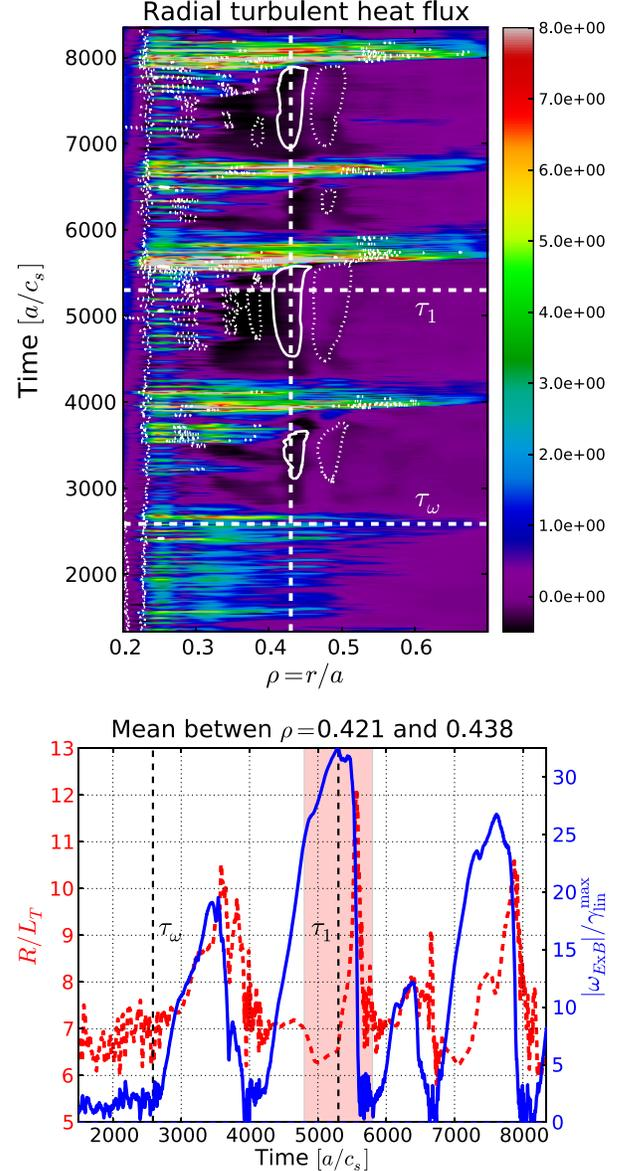
FIG. 2 (color online). Top. Turbulent heat flux (color map) and  $E \times B$  shearing rate contours (white contours: the dotted contour is  $8\gamma_{\text{lin}}$ , and the plain contour is  $-20\gamma_{\text{lin}}$ ). Bottom.  $E \times B$  shearing rate  $\omega_{E \times B}$  (plain blue line) and temperature gradient  $R/L_T$  (dashed red line) radially averaged close to  $\rho_\omega$ . The red area corresponds to the zoom window used in Fig. 3.
