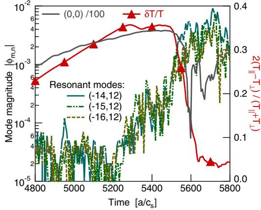
FIG. 3 (color online). Time evolution of the local resonant Fourier  $(m, n)$  modes left to the TB ( $\rho = 0.41$ ), during the second quenching. The temperature anisotropy is displayed in thin black line.
