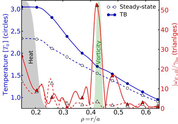
FIG. 1 (color online). Temperature (blue circles) and  $E \times B$  shear (red triangles) during steady-state (open) and a TB phase (solid). The kinetic sources are labeled by the black and green areas.
