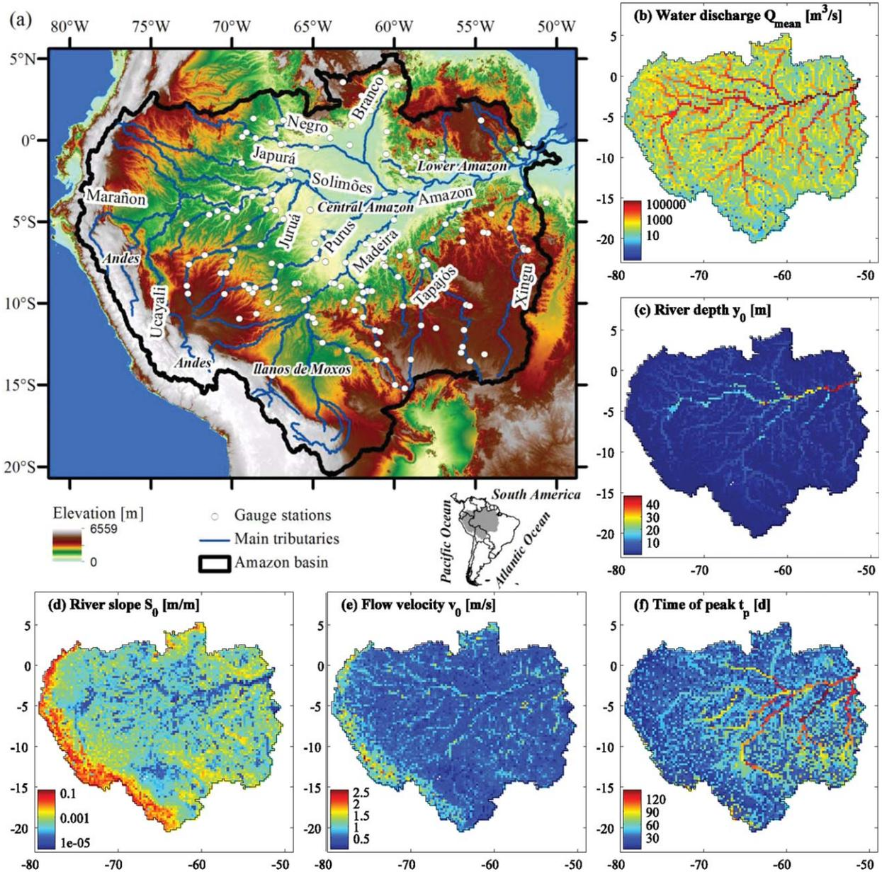
**Figure 2.** The Amazon Basin: (a) main tributaries and stream gauges (white dots), (b) mean discharge ( $Q_{\text{med}}$ ), (c) river depth ( $y_0$ ), (d) local surface water slope ( $S$ ), (e) mean flow velocity ( $v_0$ ), and (f) time to peak ( $t_p$ ).
