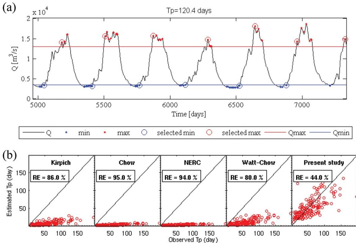
**Figure 3.** Time-to-peak ( $t_p$ ) calculation: (a) example of the automated method to define observed  $t_p$  from hydrographs and (b) comparison of estimated and observed time-to-peak values derived from different equations.
