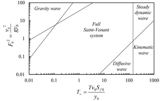
**Figure 1.** Criteria for flood wave type classification from *Moussa and Bocquillon* [1996].
