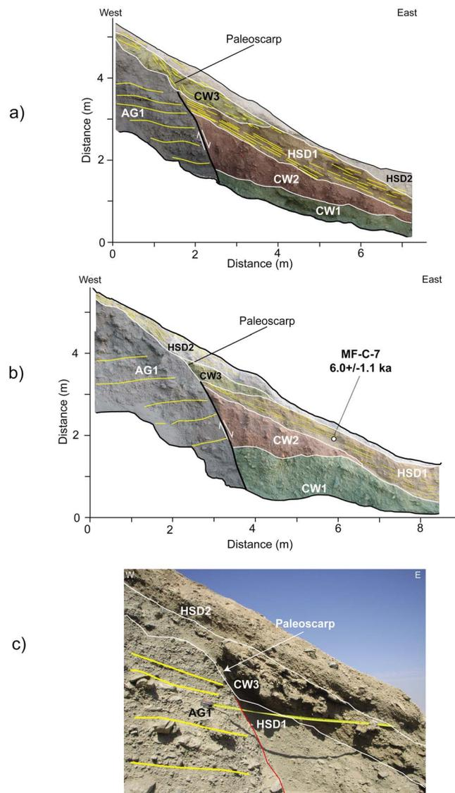
**Figure 11.** (a) Log of trench C, northern wall. (b) Log of trench C southern wall. Samples sites for OSL dating method are depicted by white circles in trench logs. (c) Picture showing the paleoscarp and CW3 unit. AG1: alluvial gravels. CWD1, CW2 and CW3: colluvial wedge deposits. HSD1 and HSD2: hillslope deposits.
