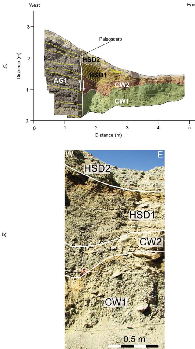
**Figure 12.** (a) Log of trench D northern wall. (b) Picture showing the red horizon between CW1 and CW2. Also, the contact between HSD1 and HSD2 is depicted. AG1: alluvial gravels. CW1 and CW2: colluvial wedge deposits. HSD1 and HSD2: hillslope deposits.
