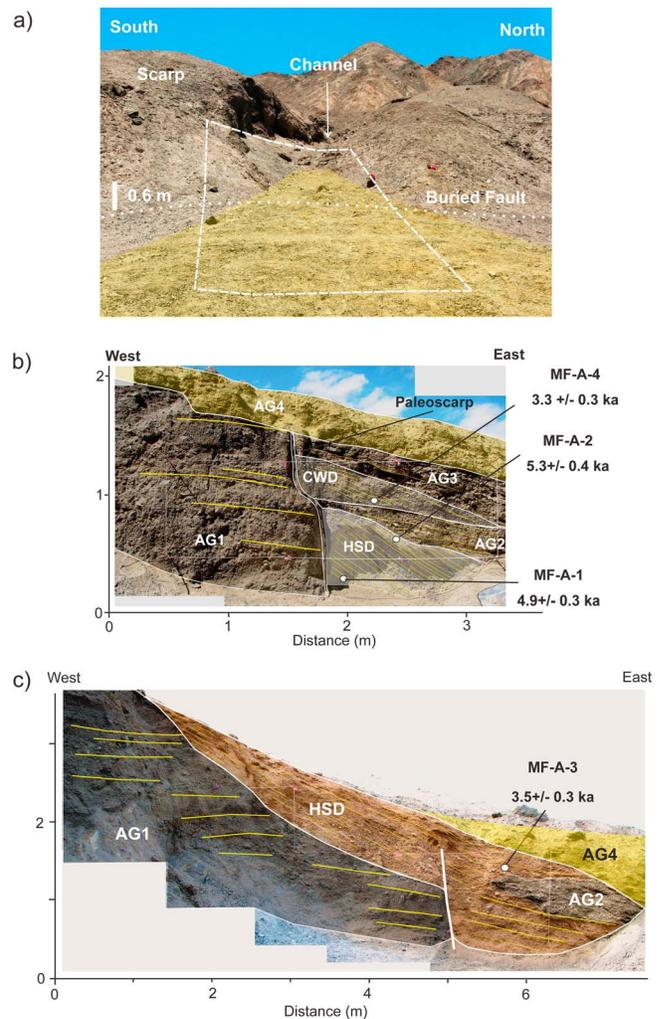
**Figure 9.** (a) Shows the trench A site. (b) Log of trench A, northern wall. (c) Log of trench A southern wall. White circles in trench logs depict location of samples for OSL dating method. AG1 to AG4: alluvial gravels from older to younger. CWD: colluvial wedge deposit. HSD: hillslope deposit.
