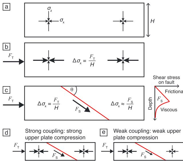
**Figure 6.** Sketch illustrating the concept of plate coupling.  $\sigma_x$  and  $\sigma_z$  are the horizontal stress and vertical stress, respectively.  $F_T$  is a tectonic force laterally applied to a lithosphere of thickness  $H$ .  $\Delta\sigma_x$  is the average differential stress resulting from the force  $F_T$ .  $F_S$  is the plate coupling force and, that is, the integrated shear stress along the fault dipping at angle  $\theta$ . See text for details.
