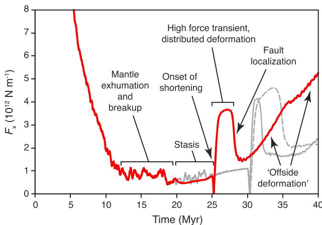
**Figure 9.** Temporal evolution of the horizontal force  $F_X$  applied to extend or shorten the model at a given rate. Red line is for the reference model (20-Myr rifting followed by shortening at a rate of 4 mm/year), gray solid line for alternative model 1 (25-Myr rifting, 4 mm/year shortening), and gray dashed line for alternative model 2 (25-Myr rifting, 2 mm/year shortening).
