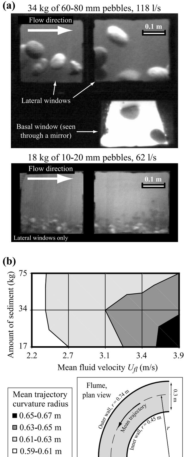
**Figure 2.** (a) Snapshots of movies recorded with a high speed camera to track the trajectories of pebbles in saltation during experiments with (top) 34 kg of 60–80 mm pebbles and an input discharge of 118 l/s and (bottom) 18 kg of 10–20 mm pebbles and an input discharge of 62 l/s. (b) Mean trajectory curvature radius as a function of fluid velocity and sediment amount for the 60–80 mm pebbles. Trajectories with large curvature radius are observed for high velocity and low sediment.
