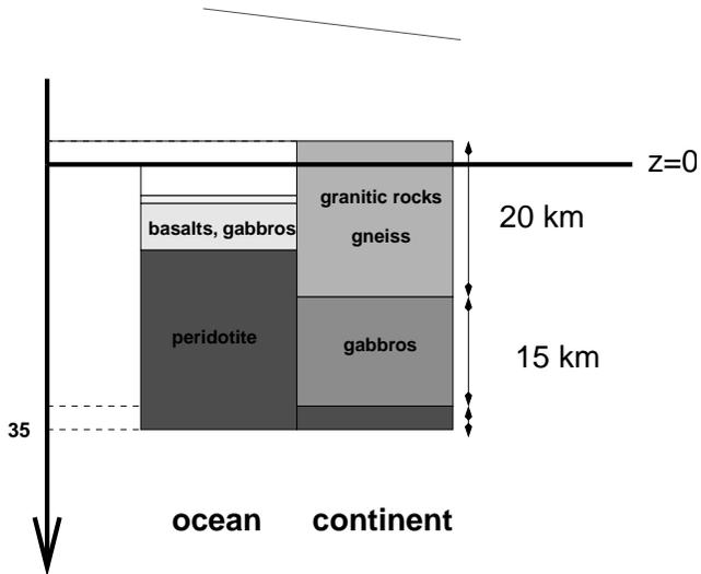
Figure 11. Simple model of continental and oceanic crust.
