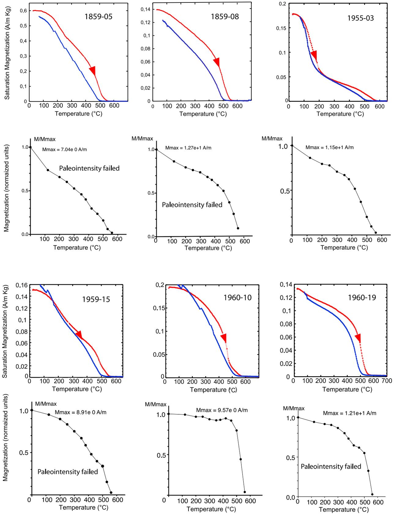
**Figure 1.** Typical thermomagnetic curves for samples from the 1859, 1955 and 1960 Hawaiian flows. For each sample is shown the evolution of the initial NRM of a companion sample taken from the same core as a function of temperature. The changes in NRM have been derived from the experiments of absolute paleointensity. Samples that did not yield any suitable result are mentioned as failed, while all others have been successful.
