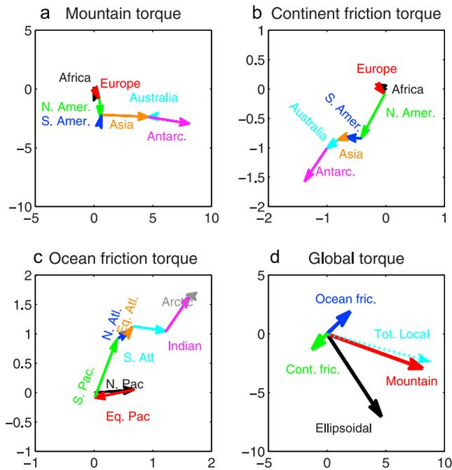
**Figure 4.** Phase diagram of the covariance of the local torque with the SOI, by (a and b) continent and (c) ocean basin, and of (d) the total local and ellipsoidal torques. Units are  $10^{18}$  Nm, with the  $X$  and  $Y$  components given by the horizontal and vertical axes, respectively. Note that the scales are different for each graph.
