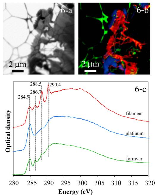
**Figure 6.** STXM analysis of FIB foil B at the C K-edge. (a) STXM image of the organic filament on FIB foil B at 288.7 eV. (b) Composite map obtained by overlaying the maps of carbon composing the filament (red), map comprising the platinum strap (blue) and carbon composing the lacey formvar (green). (c) NEXAFS spectra at the C K-edge of the filament, the platinum strap, and formvar.
