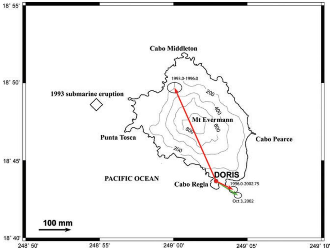
**Figure 6.** Cumulative displacements of the DORIS station observed between 1993.0 and 1996.0, between 1996.0 and 2002.75 and almost instantaneously on 2003 October 3.
