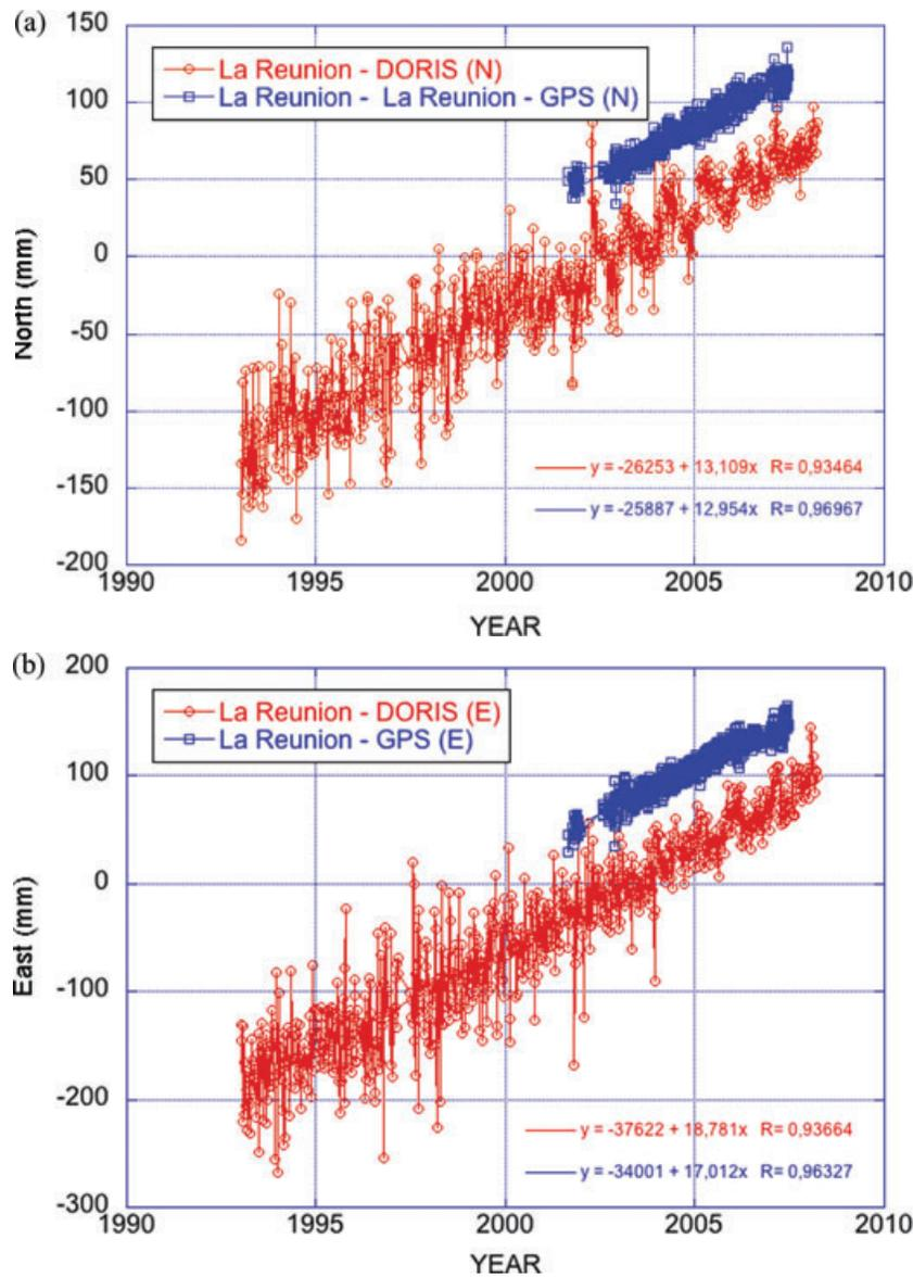
**Figure 3.** (a) Northward velocity of La Reunion DORIS (red) and GPS (blue) stations. Both are located at a few metres distance at the Piton de la Fournaise volcano observatory. (b) Eastward velocity of La Reunion DORIS (red) and GPS (blue) stations.
