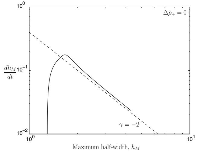
**Figure 9.** Time rate of change for the maximum width of a dike that penetrates into a layer with neutral buoyancy. Dashed line: power law relationship deduced from a simple local hydrostatic model (see text, equation (27)).
