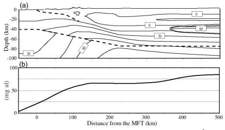
Figure A2. (a) Density variations resulting from thermal expansion and bulk modulus of rocks (isovalues in kg m<sup>-3</sup>). This computation corresponds to the end-member case when crustal rocks are given a granite-type thermal expansion coefficient (see Appendix A). (b) Gravity corrections implied by (a) are as high as 80 mgal under southern Tibet.
