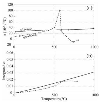
Figure A1. Empirical measurements of thermal expansion, as a function of temperature, for granite (Jeanloz & Knittle 1986) and olivine (Chayé d'Albissin & Sirieys 1989). (b) Temperature-integrated form of the thermal expansion coefficients in (a).
