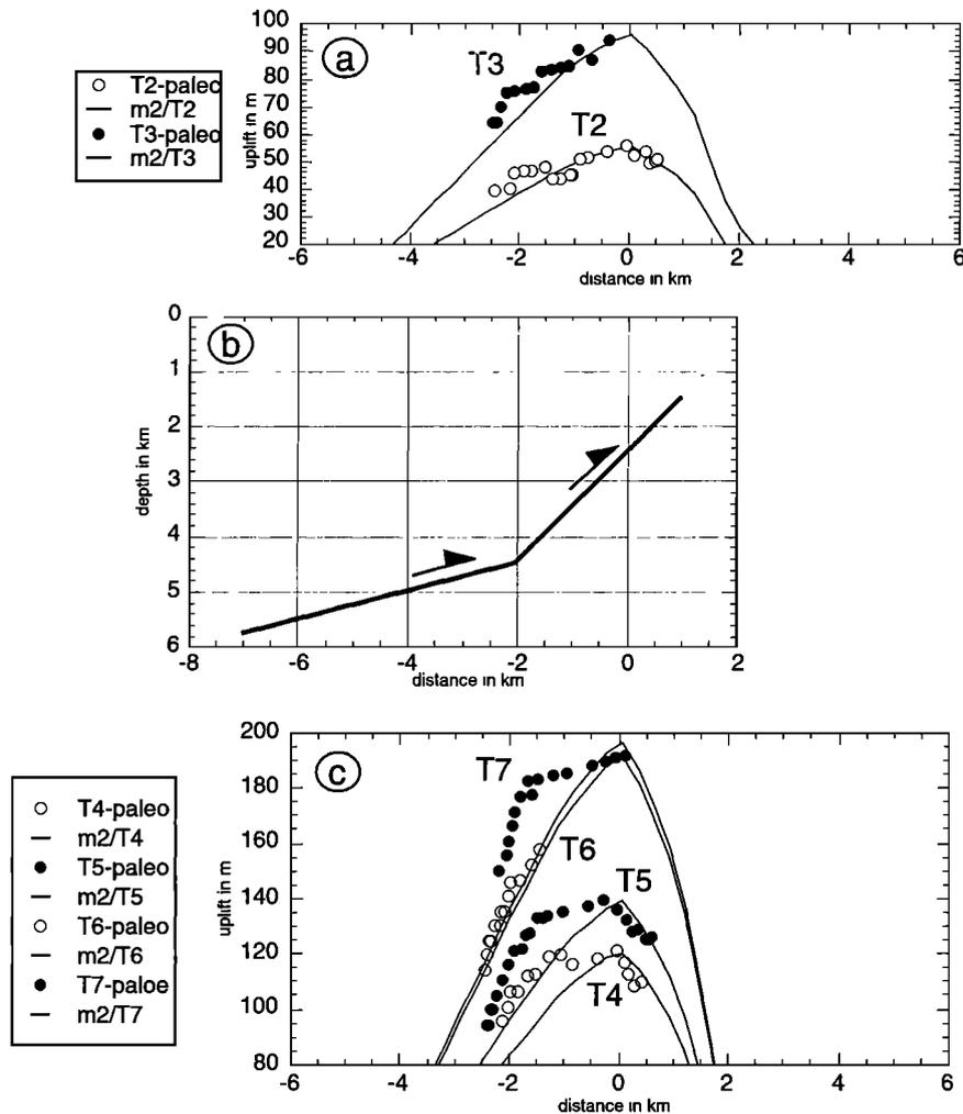
**Figure 9.** (a) Same as figure 8 with paleovalley shape subtracted (data, circles, and model, lines). (b) New geometry of fault used to model T2 and T3 (m2). Top of ramp is 1.5 km from surface. The 4.2-km-long ramp dips 45°N to meet same low angle thrust at same depth as in m1. (c) Fit is still poor with T4 to T7 profiles.
