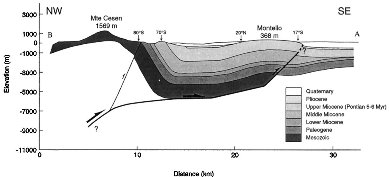
**Figure 3.** Geological cross section of Montello anticline (see location on Plate 2b) from Dal Piaz et al. [1963], Pieri and Groppi [1981], Slejko et al. [1987] and our observations. Topography is from IGM [1950] and is shown with no vertical exaggeration. Bedding dips are from field measurements.
