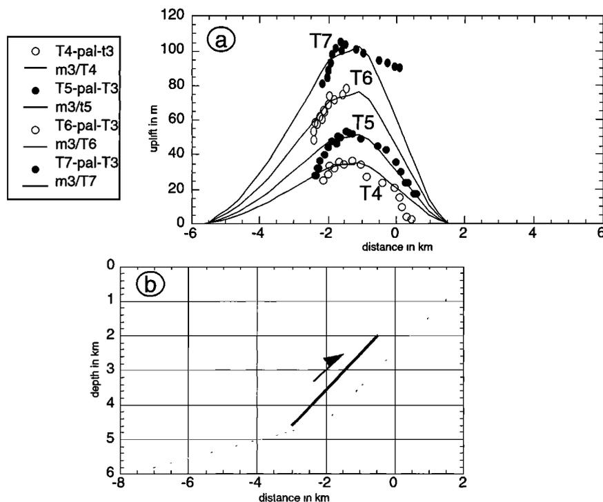
**Figure 10.** (a) Same as Figure 8 with paleovalley and T3 shape subtracted (data, circles, and model, lines). (b) New geometry of fault used to model T4 to T7 (m3). Top of ramp is 2 km below surface. Thrust ramp is 3.5-km-long and dips 45°N.
