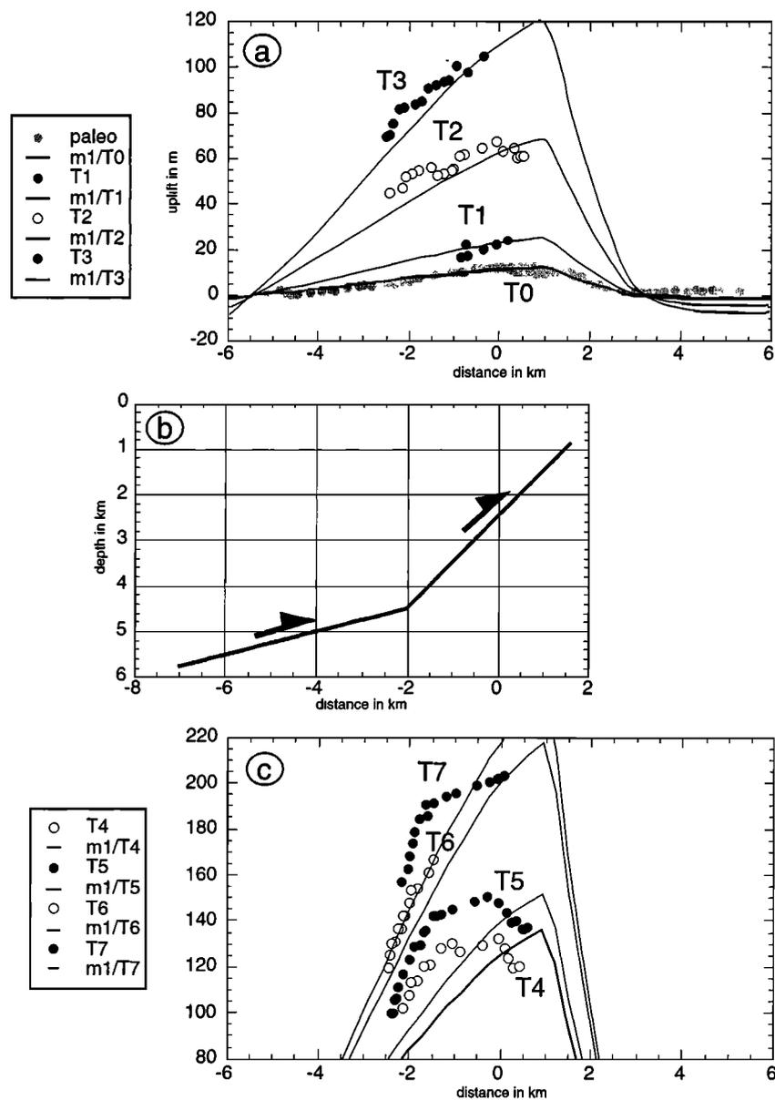
**Figure 8.** Modeling of terrace folding. (a) Profiles of paleovalley and terrace risers tops (data, circles, and model, lines). (b) Geometry of fault used to model paleovalley (m1). Top of thrust ramp is 0.9 km from surface. The 5-km-long ramp dips 45°N to meet the 5-km-long, 12°N dipping low-angle thrust 4.5-km below surface. (c) Model in Figure 8b provides fit to T4 to T7 profiles.
