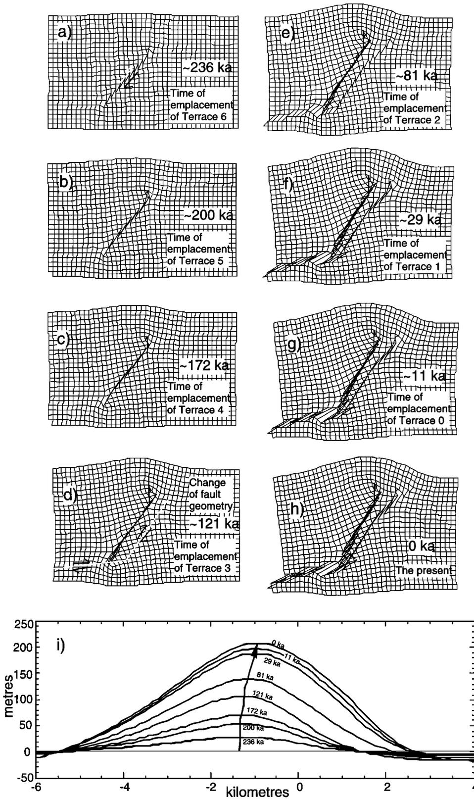
**Figure 11.** (a)-(h) Evolution of Montello anticline shape in steps corresponding to emplacement of terraces T7 to T0. No vertical exaggeration. Fault slip is 5 times actual slip. (i) Progressive modeled folding from T7 to T0. Vertical exaggeration is 10.
